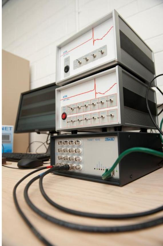
**Figure 13.** Data acquisition (bottom box) with 12 and 4 channel pre-amplifiers (middle and top boxes, respectively).
