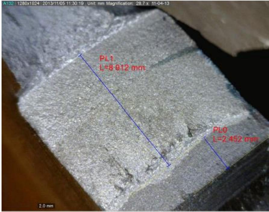
Figure 16. Specimen 1 crack length measurements from microscope.
