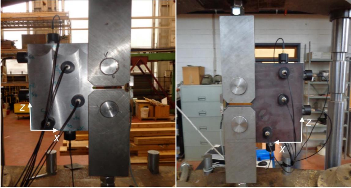
**Figure 12.** Back (left photo) and front (right photo) side of Specimen 1 with AE sensor network. The white arrows depict the coordinate system used for the sensors.
