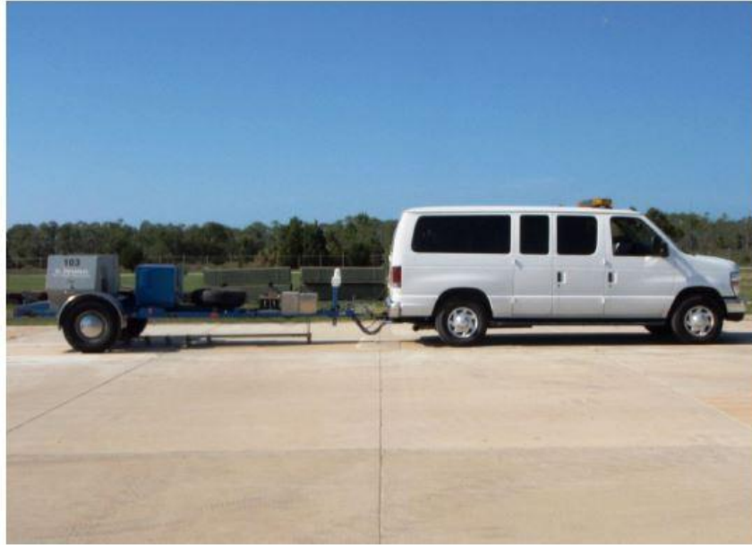
Figure – 19 Heavy Weight Deflectometer [3]
