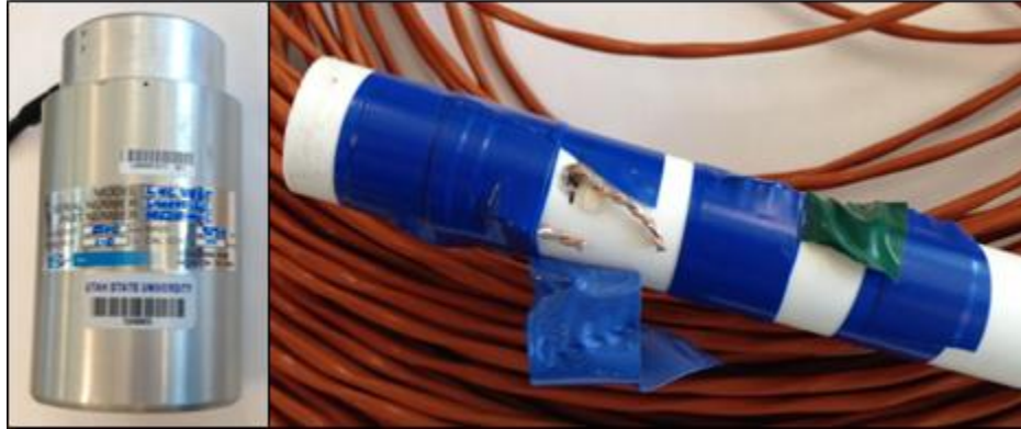
Figure 29: Uninstalled Velocity Transducer & Deck Thermocouples
