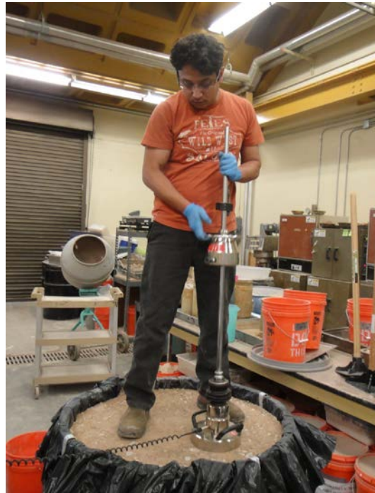
Figure 3.8 Small-scale test with LWD
