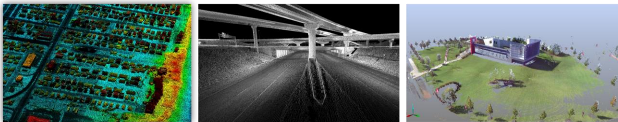
Figure 2 Lidar data comparison: (left) airborne lidar; (middle) mobile lidar; (right) static terrestrial lidar
