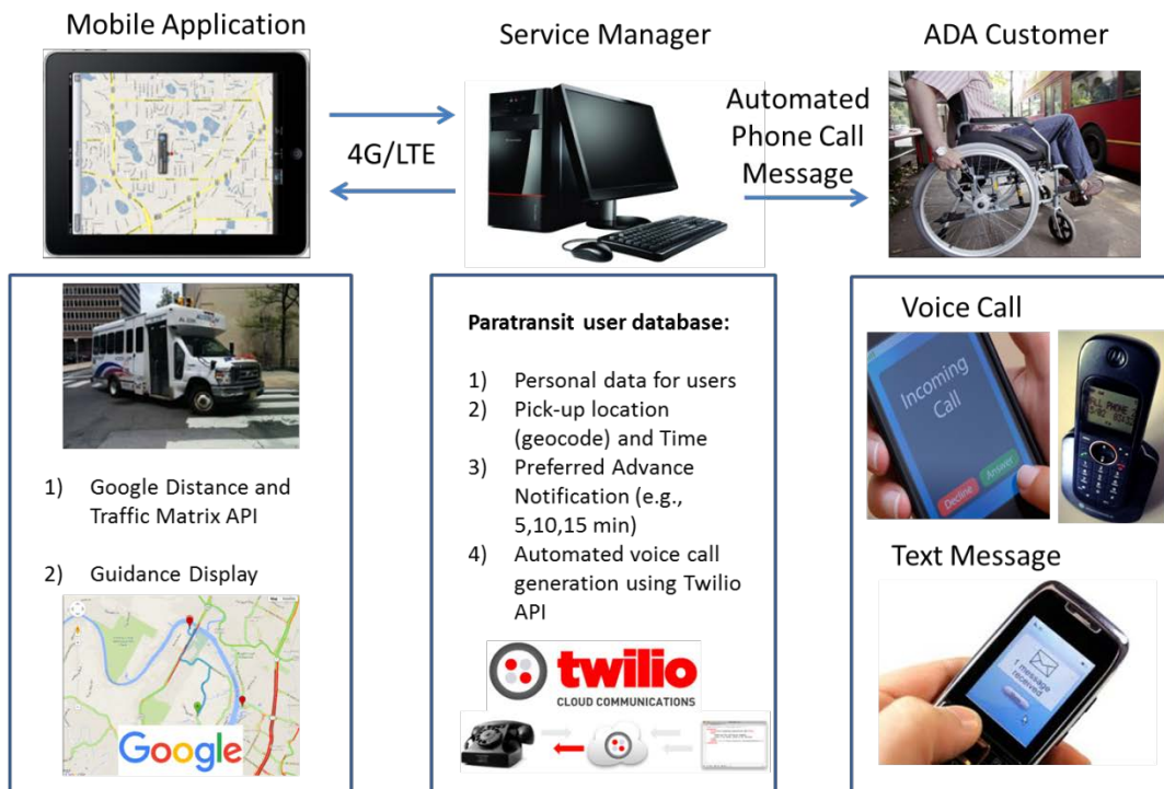
Figure 1. Passenger advanced notification- system architecture
