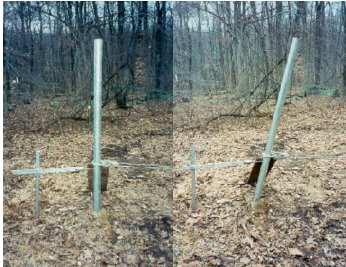
Figure 19 Testing results of Anchor Post #6 a 3 inch diameter post installed with drive anchors. Shows deformation of soil resulting in post inclination.
