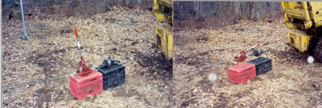
Figure 16 This figure shows a before and after picture of the ratchet and load cell. The before picture, on the left, shows the devices lying on the crates ready for testing, the after picture shows the system in tension.
