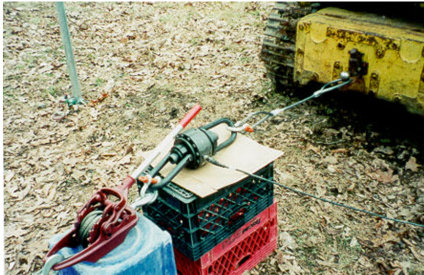
Figure 12 The testing apparatus consisting of a ratchet mechanism, load cell, and bulldozer are shown.
