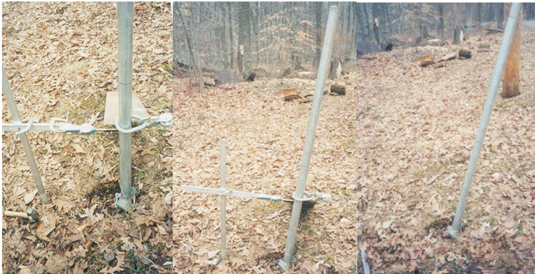
Figure 17 Testing results Anchor Post #2 of a 2.5 inch diameter line post installed with drive anchors. Shows deformation of the soil resulting in post inclination.
