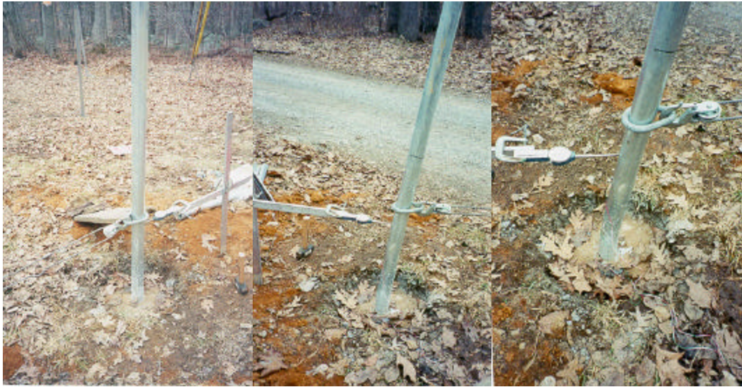
Figure 20 Testing results of Anchor Post #5 a 3 inch diameter post installed with concrete. Shows the formation of a plastic hinge in the post.
