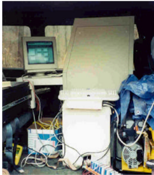
Figure 13 The data acquisition unit. The monitor shows the graphical representation of the ratchet loading.
