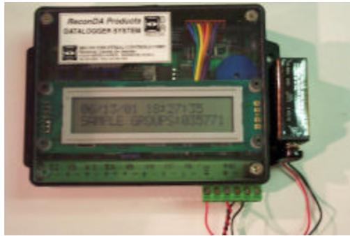
Figure 12. Data Log Module for the continuous logging of date/time stamped data.
