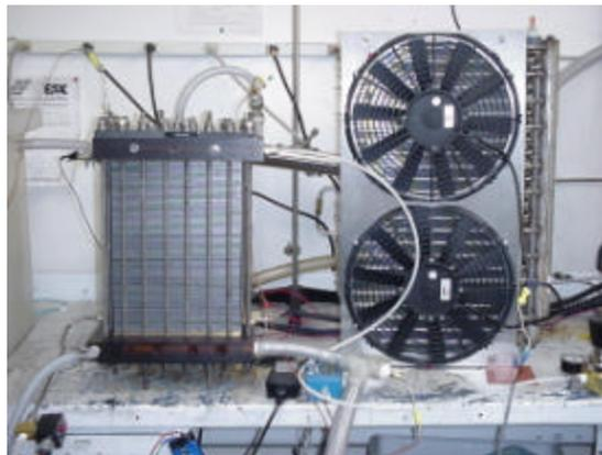
Figure 1 High-power fuel cell test stand at H-Power.
