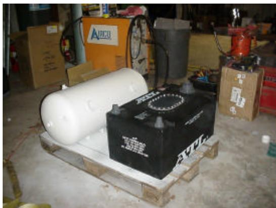
Figure 9 Spent fuel condensate / sodium borate tank (left) and fuel tank (right).
