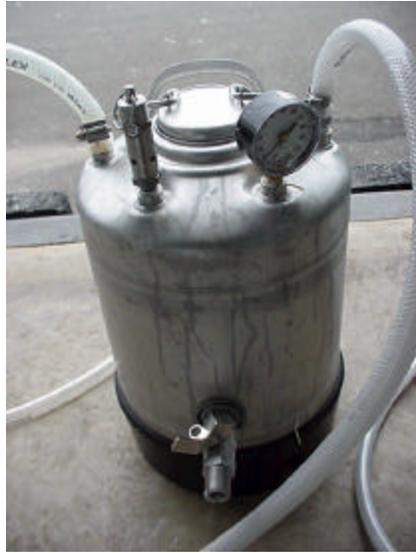
Figure 17 Hydrogen generator test stand condenser water reclamation tank used to develop hydrogen generator design prior to installation in the vehicle.
