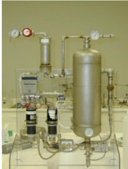
Figure 15 Millennium Cell, Inc. Hydrogen Generator Model 1 designed to power a 1.2 kW fuel cell.
