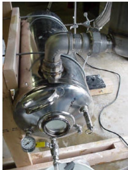
Figure 16 Millennium Cell, Inc. hydrogen generator test stand used to develop hydrogen generator design prior to installation in the vehicle.
