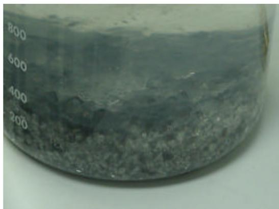
Figure 10 Crystallized sodium borate byproduct of reaction.
