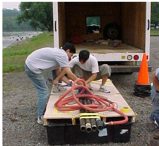
Figure 29. Floating platform used for instrumentation of Route 46 Passaic Bridge.
