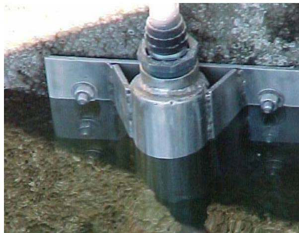
Figure 12. Sonar mounting plate as tide rises.
