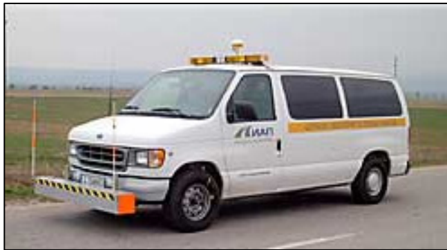
Figure 4 Dynatest Road Surface Profiler (3) .
