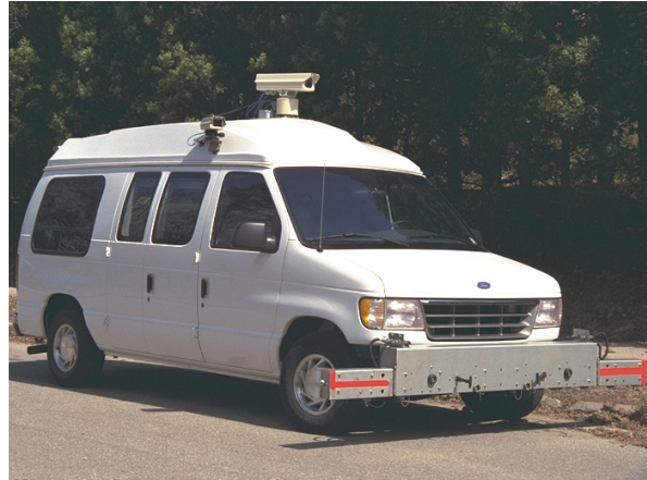
Figure 5. ICC High Speed Profiler (4) .
