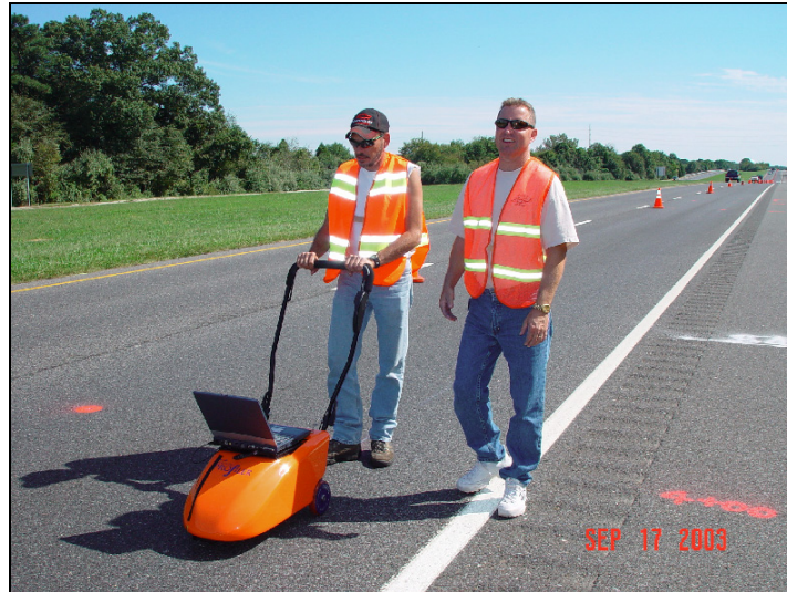
Figure 6. Field Testing with the Walking Profiler.
