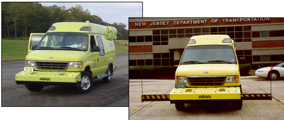
Figure 3 ARAN High Speed Profiler (2) .
