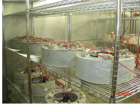
Figure 21. Close Up View of Rings in the Environmental Chamber
