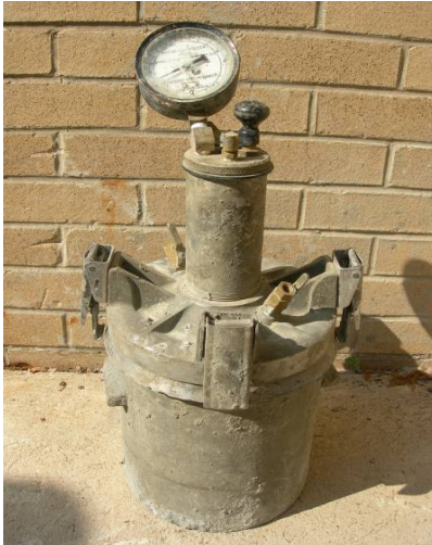
Figure 3. Type - B Pressuremeter for determining concrete air content
