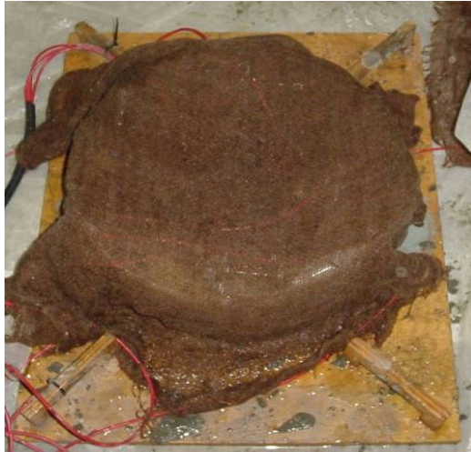
Figure 6. Restrained shrinkage specimen covered with wet burlap
