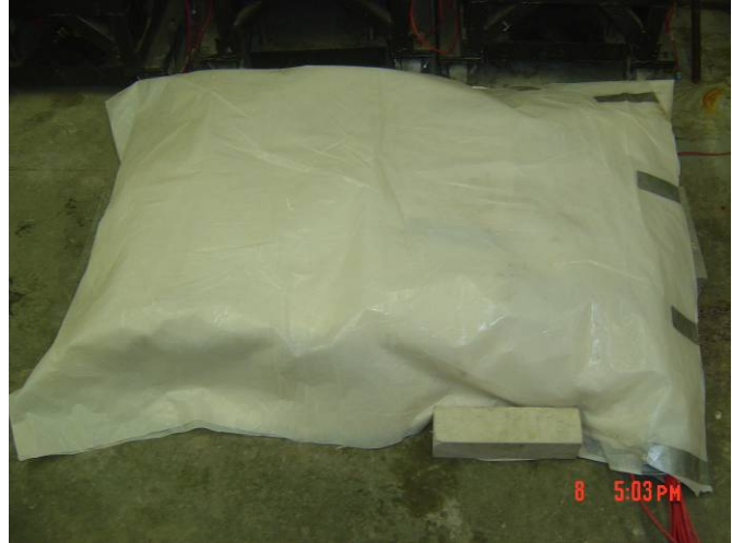
Figure 7. All Specimens Under Burlap and Polyethylene Sheet
