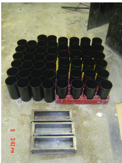
Figure 4. Shrinkage Blocks and Cylinder Molds
