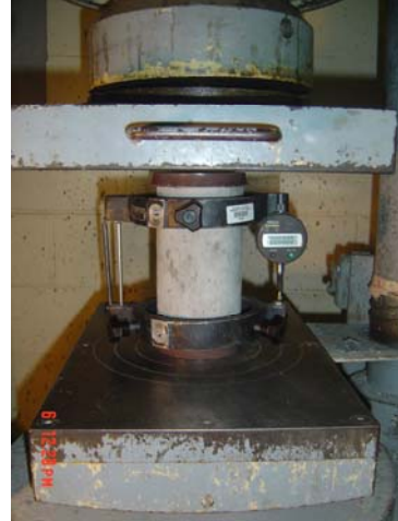
Figure 12. Modulus of Elasticity Test Setup
