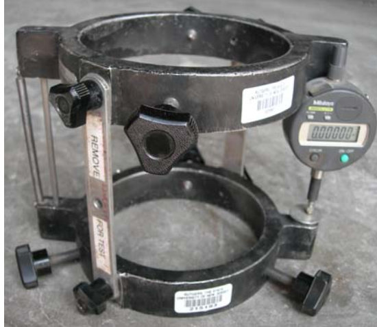
Figure 11. Compressometer used for modulus tests
