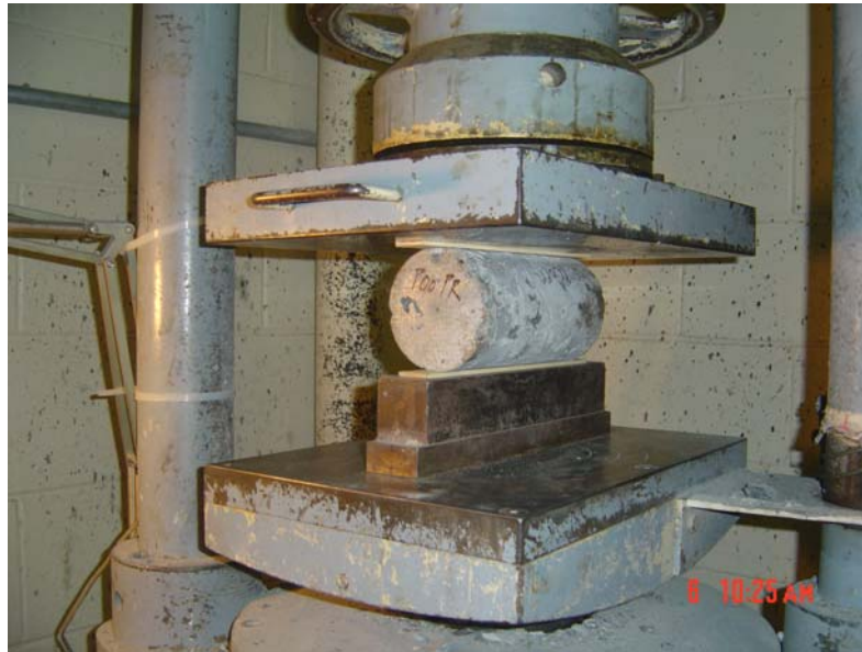
Figure 10. Splitting Tensile Strength Test Setup
