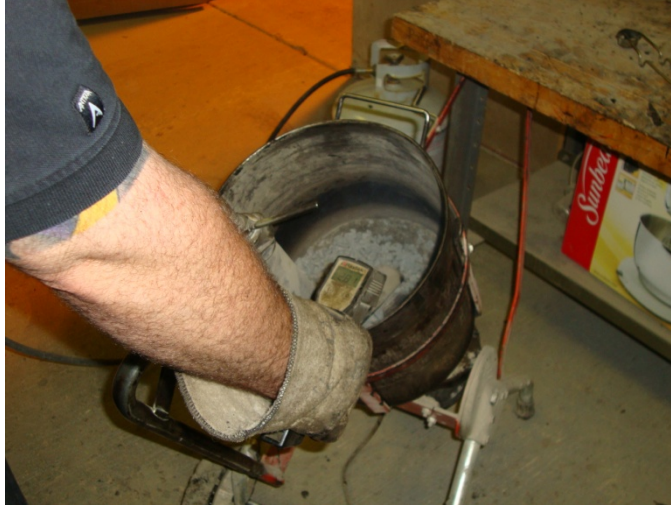
Figure 9 – Monitoring Temperature of Aggregate Blend with Infrared Temperature Probe
