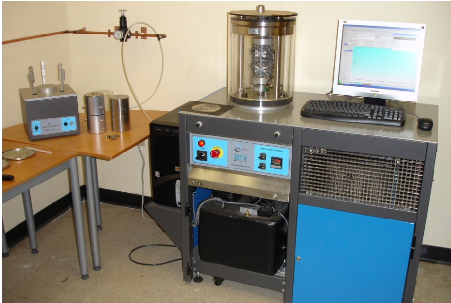
Figure 19 – Asphalt Mixture Performance Tester (AMPT) at Rutgers University
