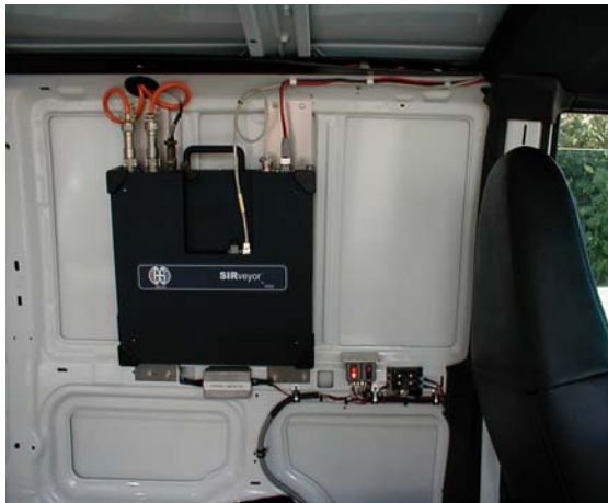
(a) SIR-20 data acquisition unit
