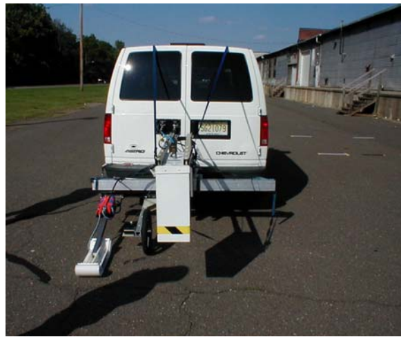
(b) Setup for network project surveys
