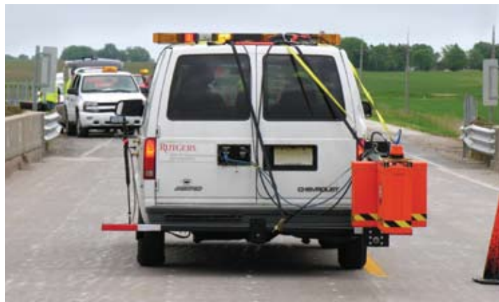
Ground-penetrating radar (above) surveys provide images of bridge decks that present an overall assessment of concrete deterioration. The Stepper (below) is a one-of-a-kind robotic device that simultaneously deploys multiple NDE technologies in one pass, in this case, impact echo and ultrasonic data. The Stepper can be expanded to incorporate other NDE technologies such as GPS, video, or radar to fill in data "gaps" other tools may not detect.
