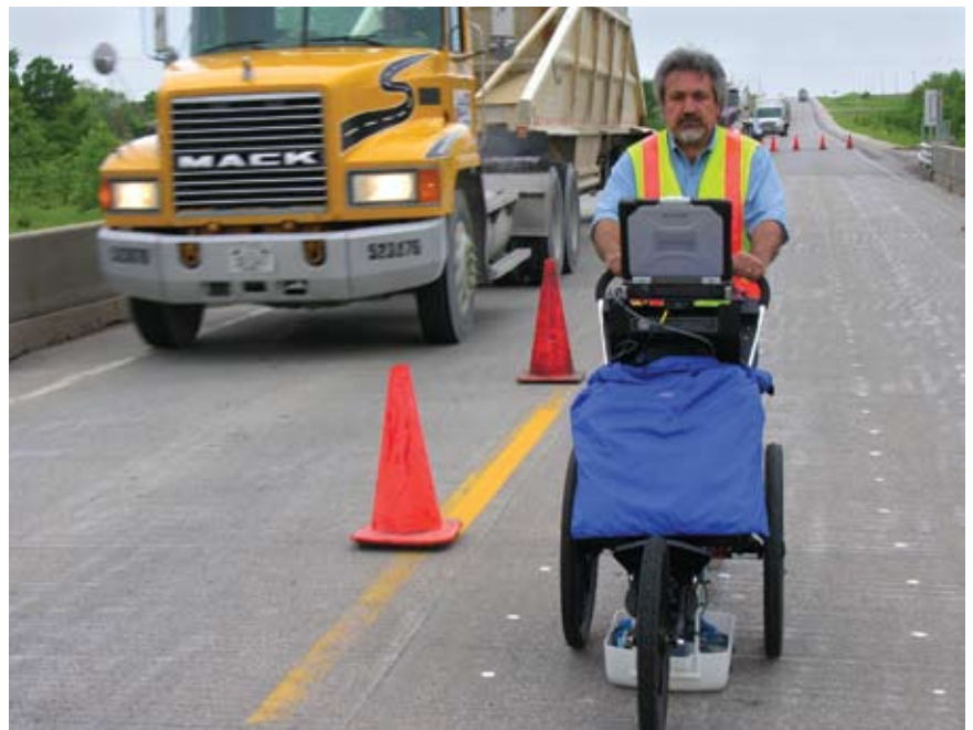
ICMP Senior Researcher Francisco Romero uses ground-coupled, ground-penetrating radar (GPR) to survey a bridge deck in Iowa. Contracted by Iowa Department of Transportation, a team of six CAIT researchers spent several weeks evaluating nine bridges in the state. A variety of NDE technologies were tested and validated to see which best suited Iowa's particular inventory and issues.
