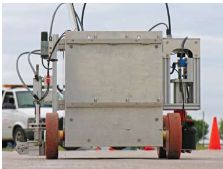
Ground-penetrating radar (above) surveys provide images of bridge decks that present an overall assessment of concrete deterioration. The Stepper (below) is a one-of-a-kind robotic device that simultaneously deploys multiple NDE technologies in one pass, in this case, impact echo and ultrasonic data. The Stepper can be expanded to incorporate other NDE technologies such as GPS, video, or radar to fill in data "gaps" other tools may not detect.
