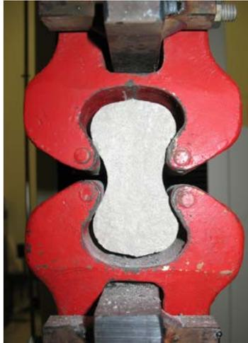
**Figure 7. Dog Bone Test Setup**
