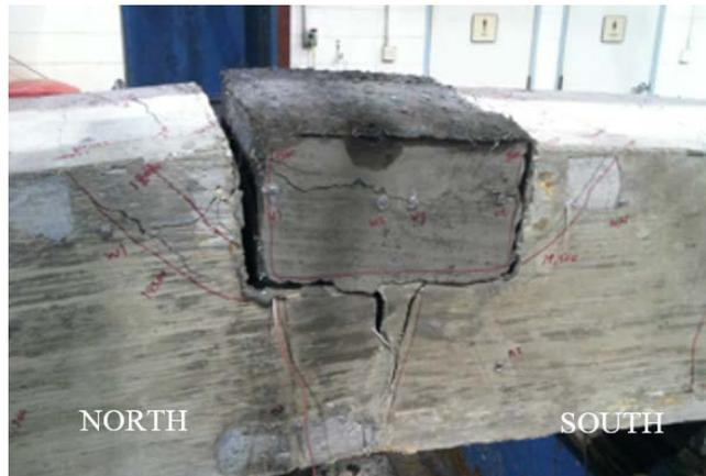
**Figure 39. VHPC Pocket in Specimen V-4-4-II Showing Interface Separation and Splitting Cracks**
