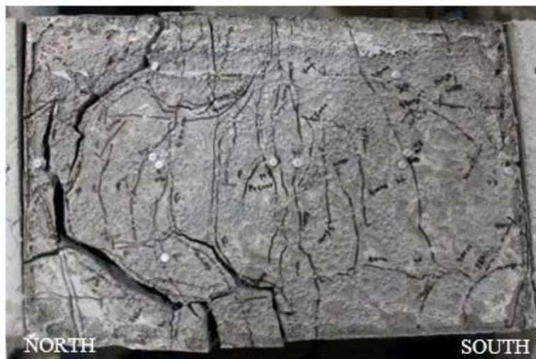
**Figure 52. Top of the UHPC Pocket in Specimen U-6-7-I After Failure**
