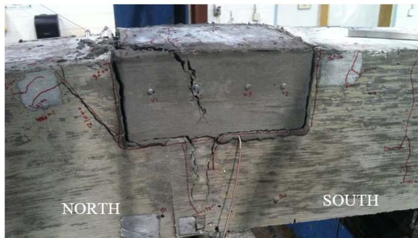
**Figure 35. VHPC Pocket in Specimen V-4-5-I Showing Interface Separation and Splitting Cracks**
