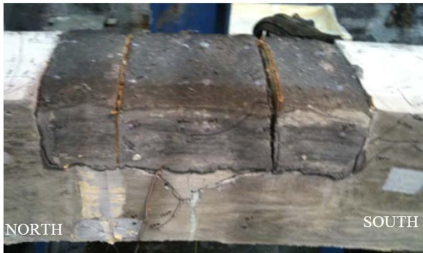
**Figure 41. VHPC Pocket in Specimen V-4-4-I at End of Load Application Showing Interface Separation**
