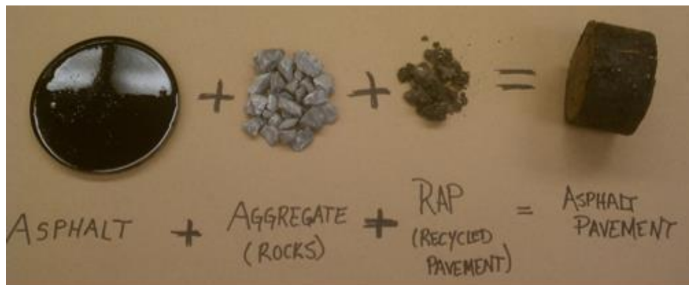
Figure A.1.5: Recycled asphalt pavement showing the virgin binder, virgin aggregate, recycled aggregate and binder, and final recycled asphalt pavement. The rejuvenators and polymer modifiers are not shown in this image, which are essential to improve the rheological characteristics of the recycled asphalt pavement (Bowers, 2016).
