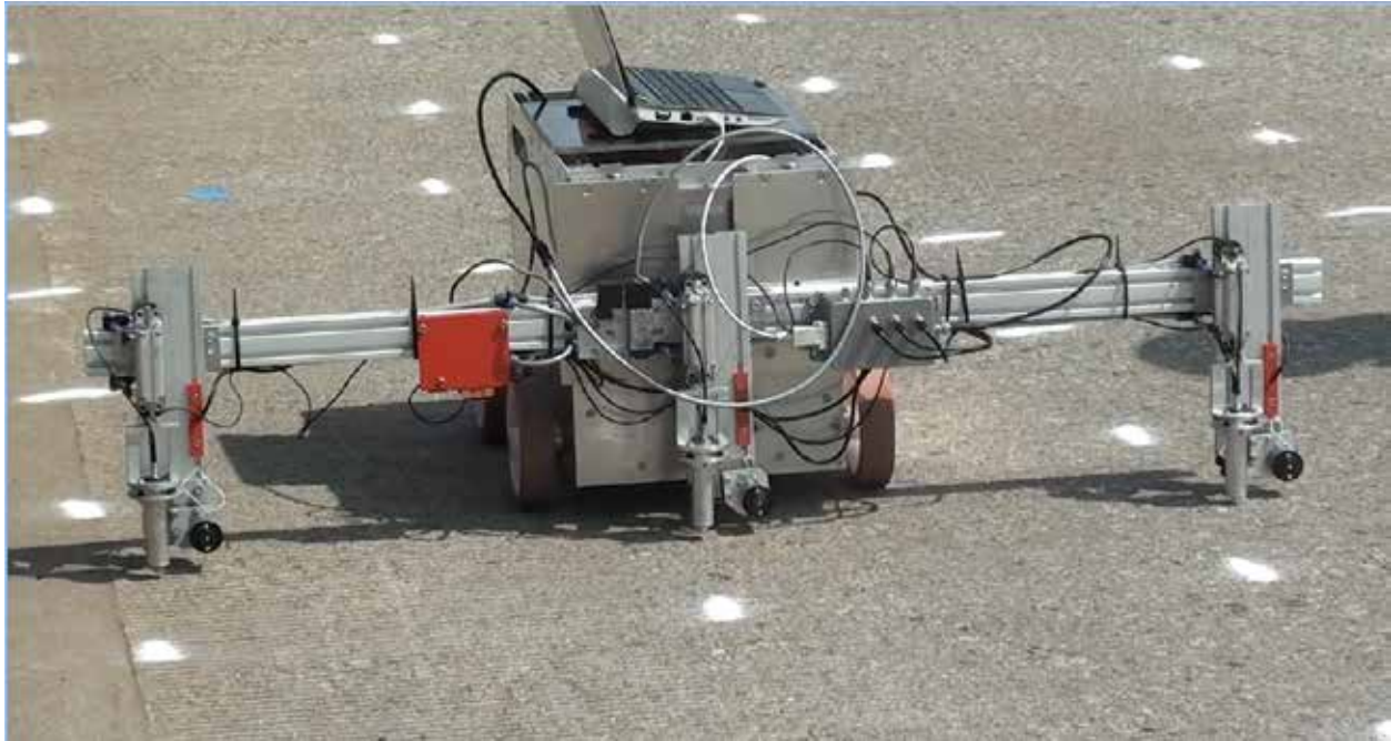
Figure A6. Delamination assessment using Stepper.
