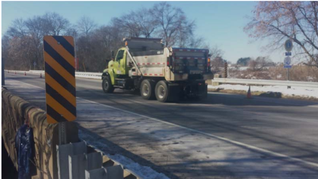
Figure 18: Truckload Test on Structure 0118150
