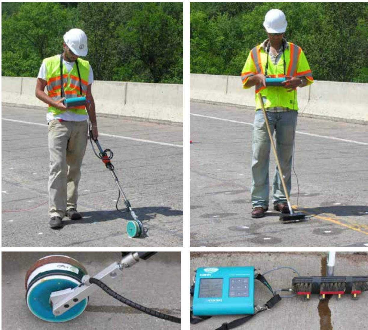
Figure A2. HCP survey using a wheel HCP probe (left) and ER survey using Wenner probe (right).
