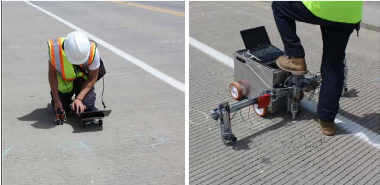
Figure 2. Impact echo testing using a single probe (left) and Stepper.
