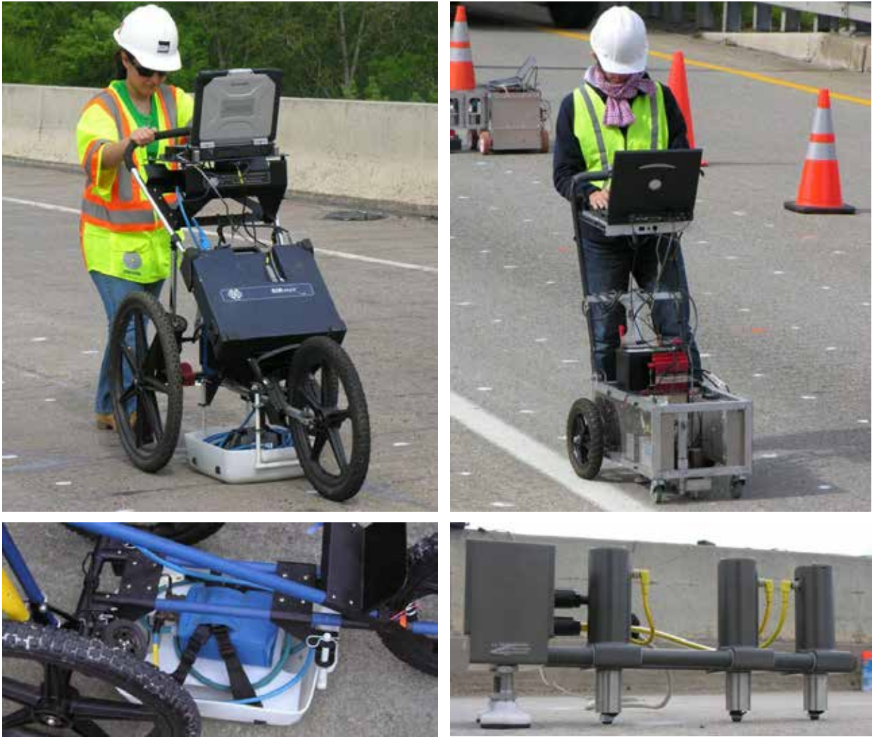
Figure A8. GPR survey using a ground coupled antenna (left) and USW testing using PSPA (right).
