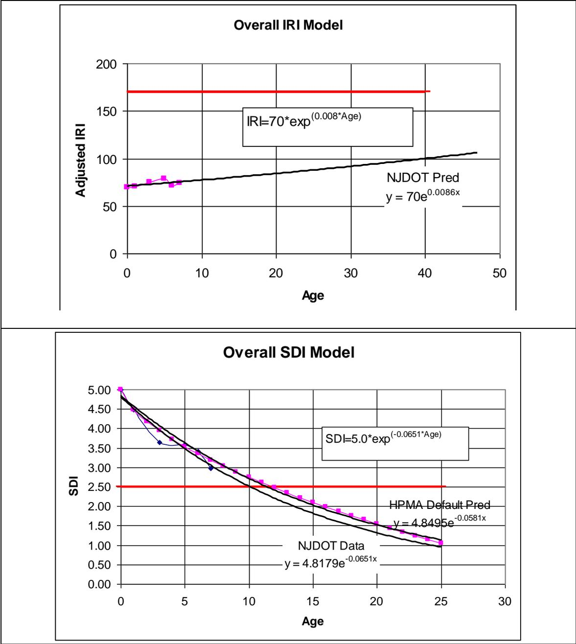
Figure 7 HMA overlay IRI and SDI pavement prediction models.
