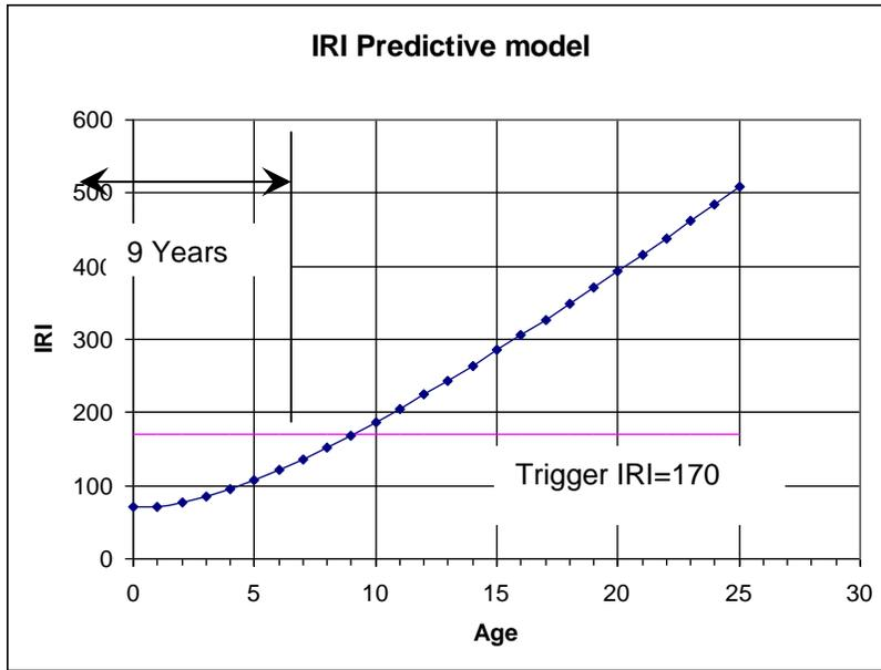
Figure 1 HPMA IRI Predictive Model for the Mill 2"/ Overlay 2" activity
