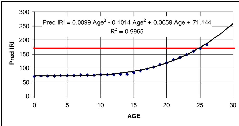
Figure 14 Recommended IRI Prediction Curve Based on SHRP LTPP data
