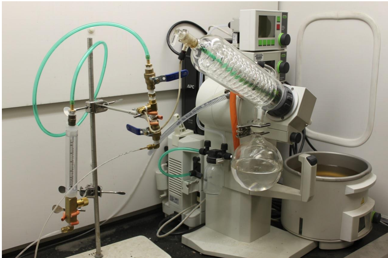
Figure 5 – Rotarvapor Solvent Extraction Set-up at Rutgers University
