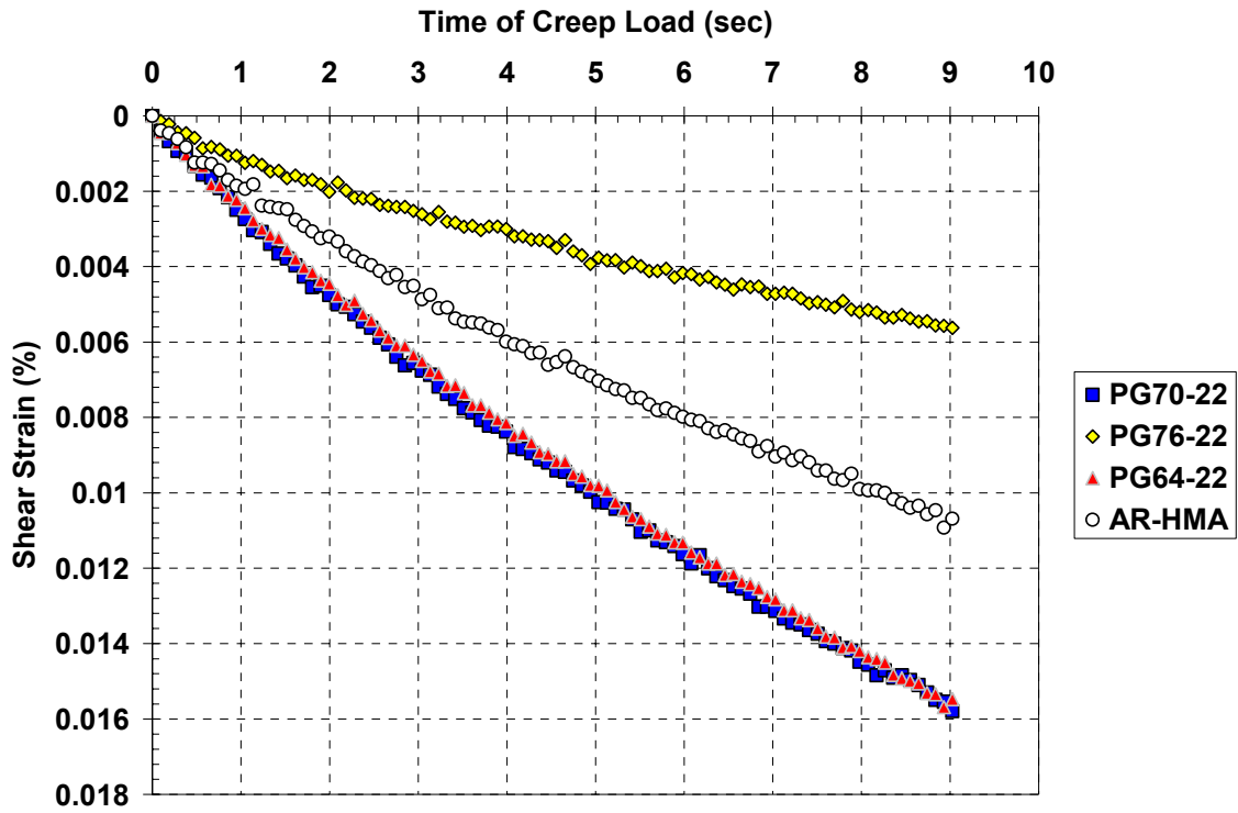
Figure 11 – SSCH Creep Slope Plots for 4°C
