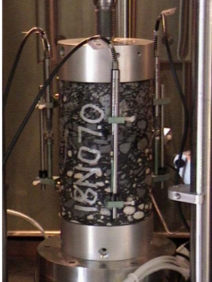
Figure 5 – HMA Sample Instrumented for the Dynamic Modulus Test
