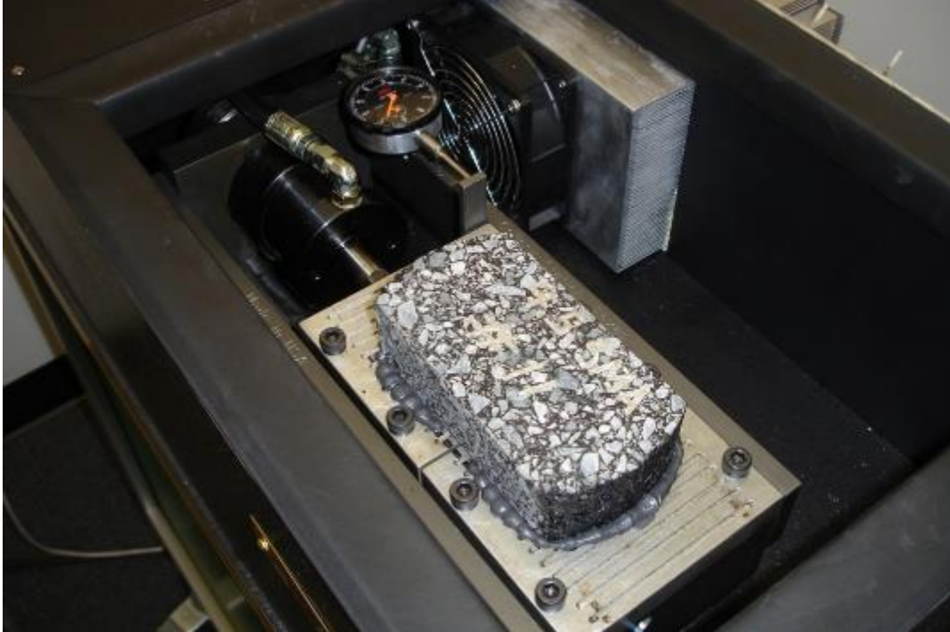
Figure 6.5 – Overlay Tester Device Used for Fatigue Cracking Assessment
