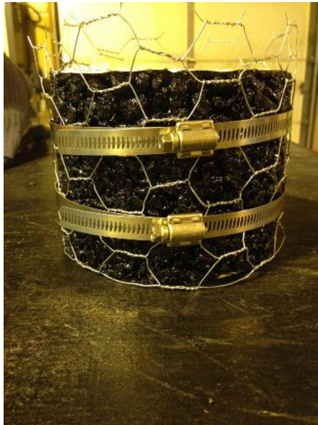
Figure 6.1 – FC-5 Specimen Confined with “Chicken Wire” Prior to Long-Term Aging
