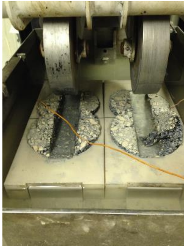
Figure 8.2 – Failed 9.5 mm NMAS FC-5 Specimens with ARB-12 Asphalt Binder
