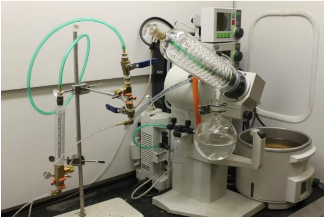
Figure 6.20 – Asphalt Binder Recovery Equipment at Rutgers University (Rotavap System)
