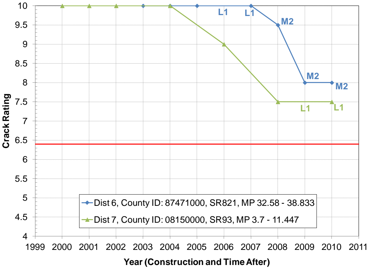
Figure 3.8 - FC-5 Cracking and Raveling Performance in District 6 and 7
