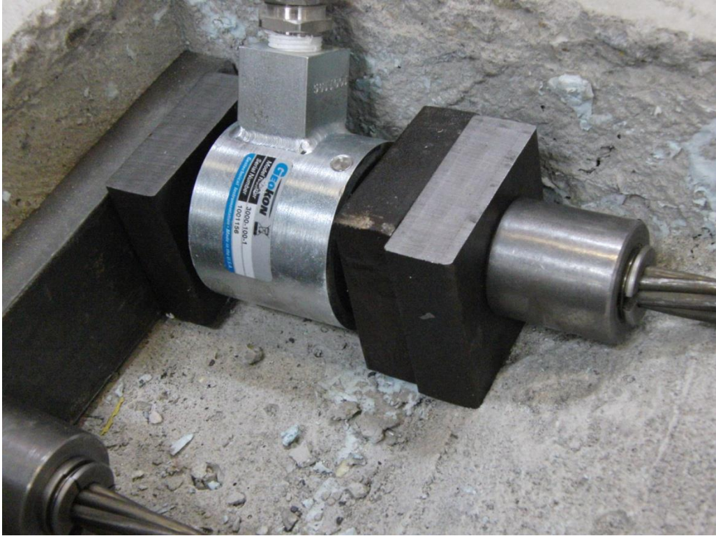
Figure 18: Load Cell on Curved Strand Connection.
