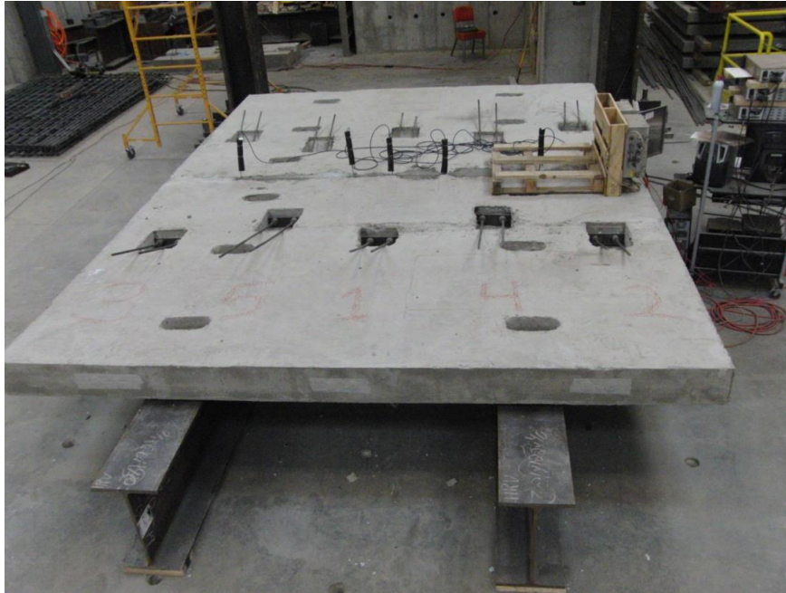
Figure 8: Layout of Full-Scale Specimen Prior to Grouting.
