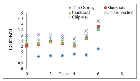
Figure 5.2 Roughness Data at Site 27 from LTPP- SPS3
