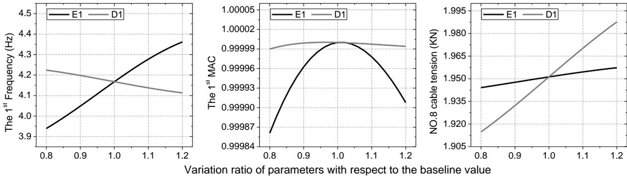
(a) The first natural frequency (b) The first MAC (c) The No. 8 cable tension
