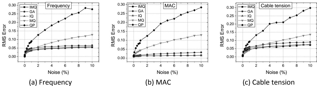
**Fig. 12.** Approximation error of RS models for frequency (a), MAC (b) and cable tension (c) under the situation of data contaminated by different degree noise
