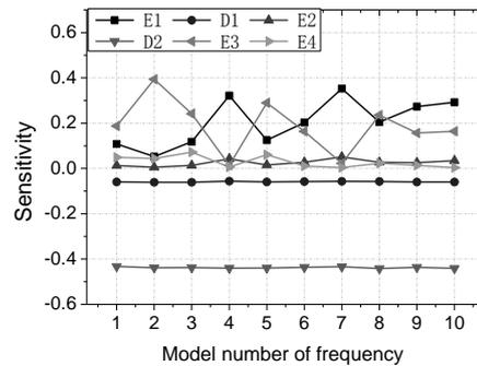
**Fig. 14.** Sensitivity of frequencies to physical parameters
