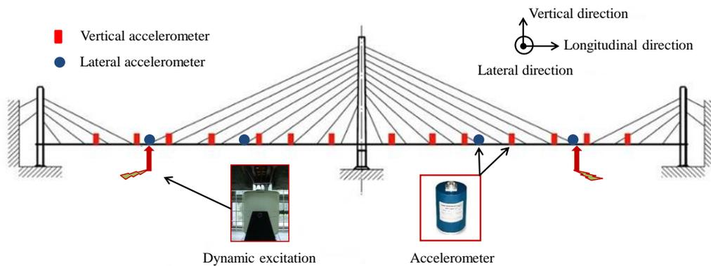
**Fig. 13.** Dynamic testing of the bridge physical model
