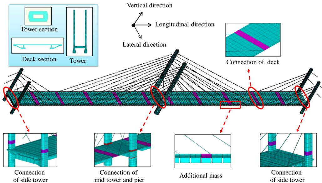
**Fig. 4.** FEM of the cable-stayed bridge model
