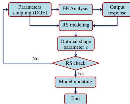
Fig. 6. The flowchart of RS modeling based on RBFs
