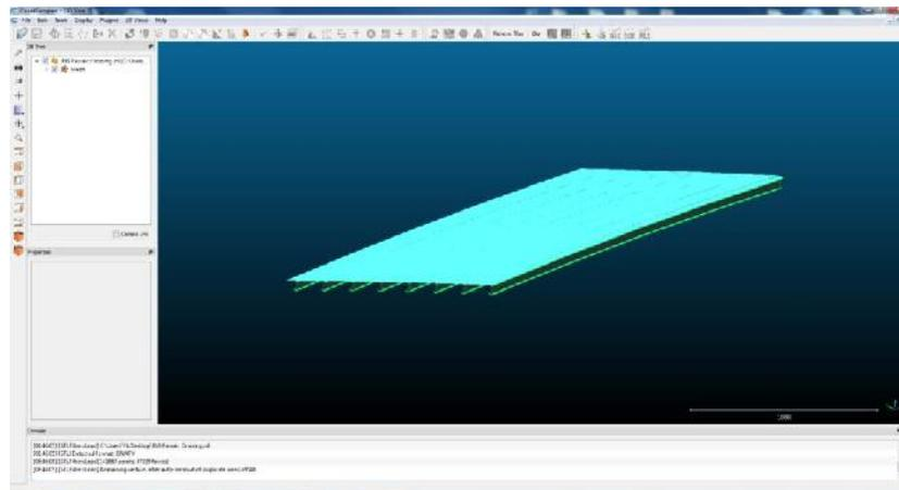
Figure 27 STL model of the bridge in CloudCompare
