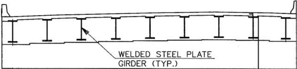
Figure 5 Typical bridge section
