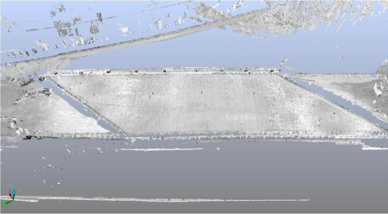
Figure 18 Point cloud for rebar surface
