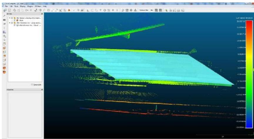
Figure 28 Difference between the aligned CAD and Point Cloud Data
