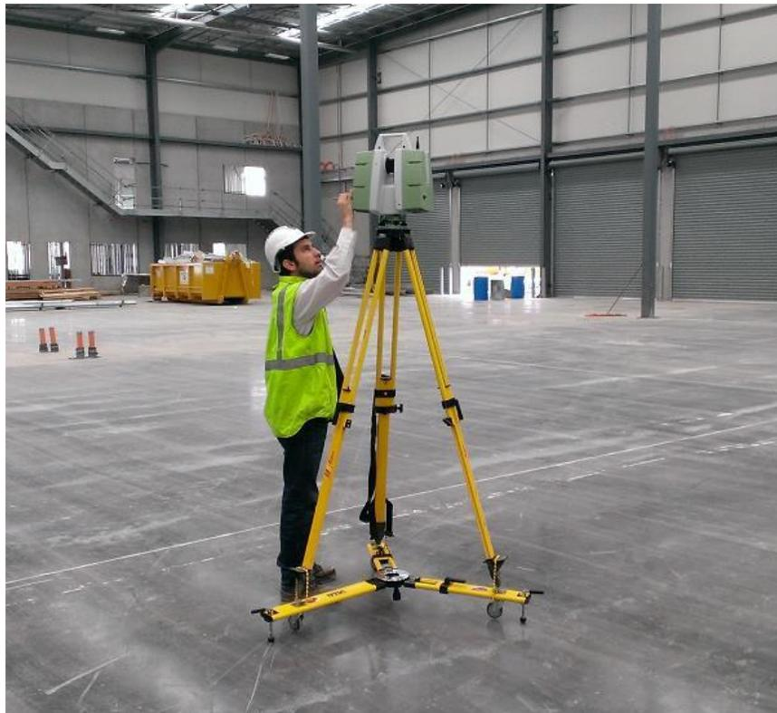
Figure 2 An example of TLS, Photo courtesy of AAM group
