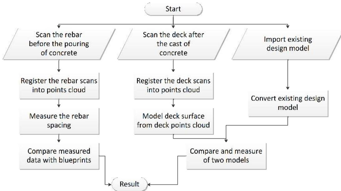
Figure 12 General workflow of bridge scan
