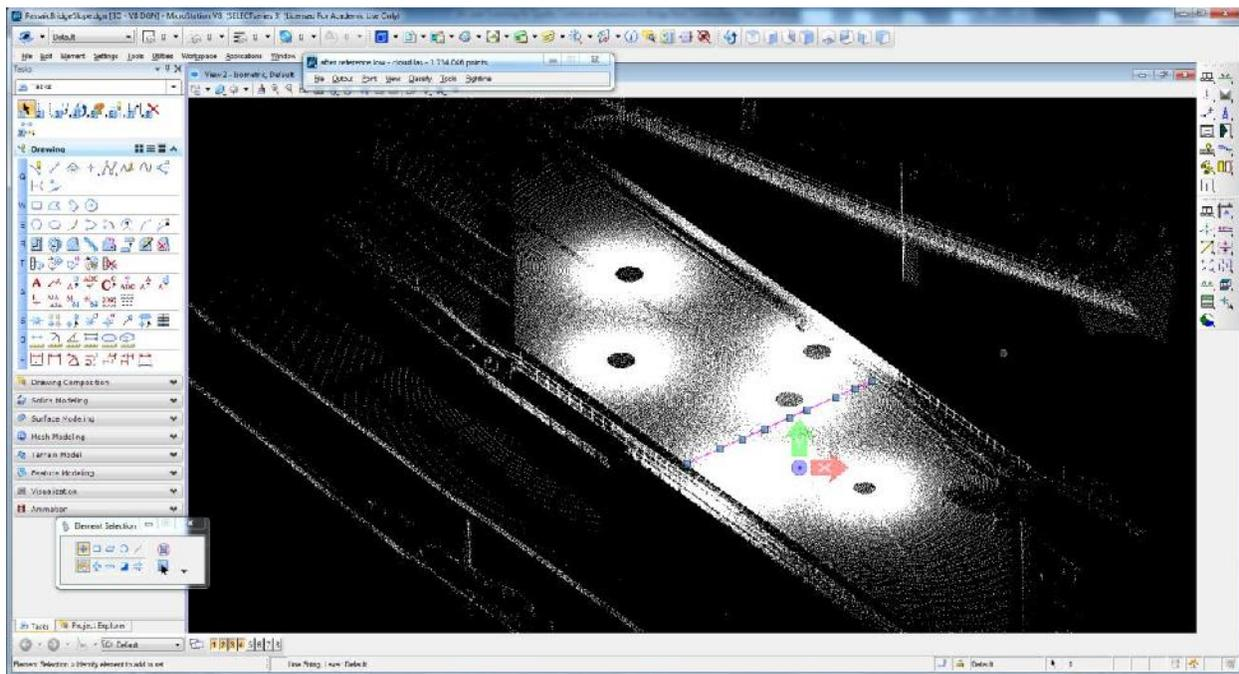
Figure 29 Measure the slope of bridge surface
