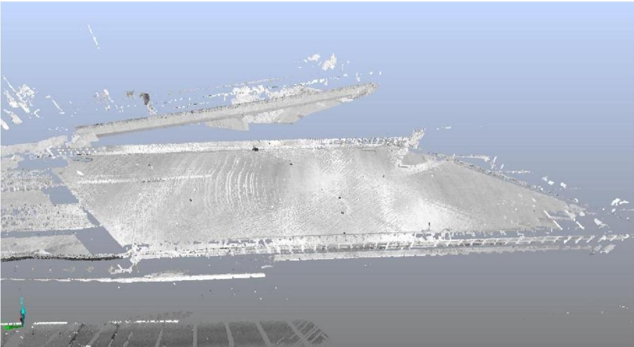
Figure 19 Point cloud for the concrete bridge surface
