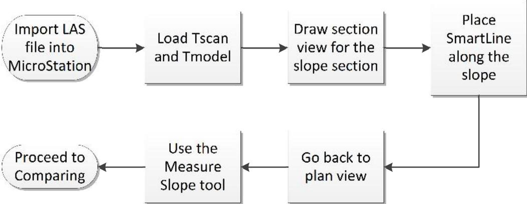
Figure 30 The slope measurement workflow
