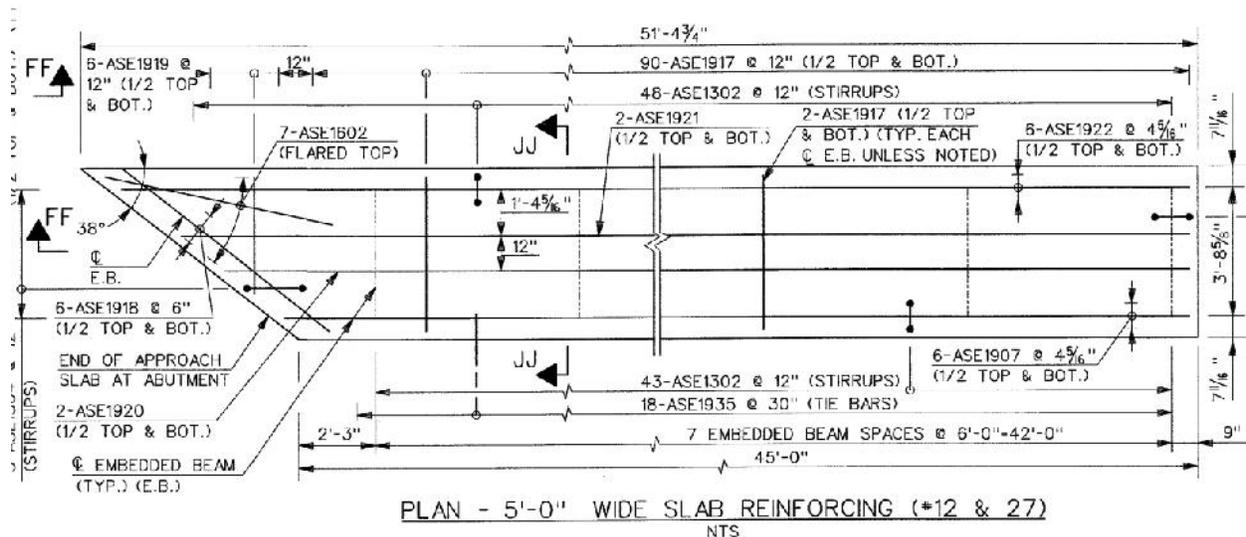
Figure 22 Rebar spacing
