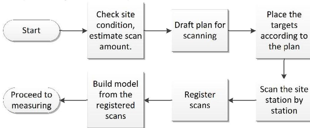
Figure 3 Typical Bridge Deck Scanning Workflow
