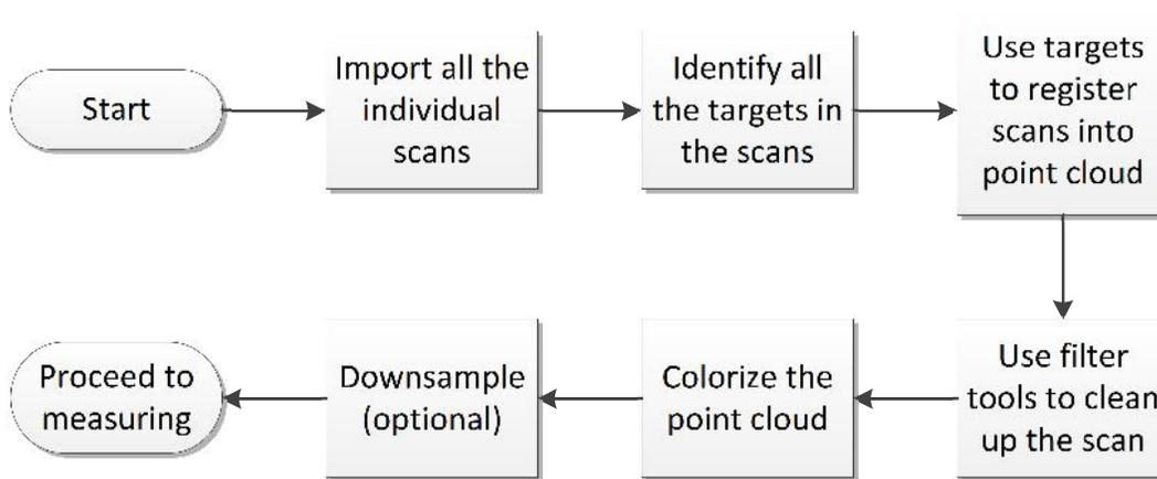
Figure 4 Bridge scans processing workflow
