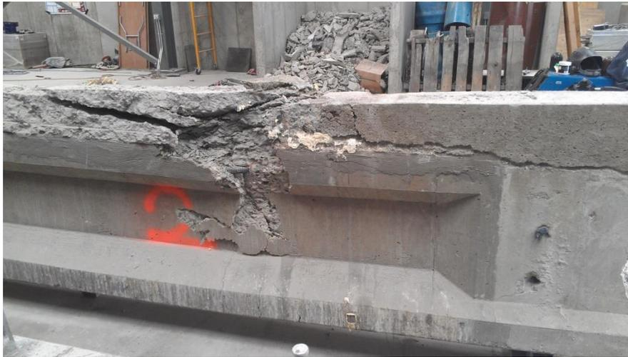
Figure 27 Compressive failure for G2-1d(a)
