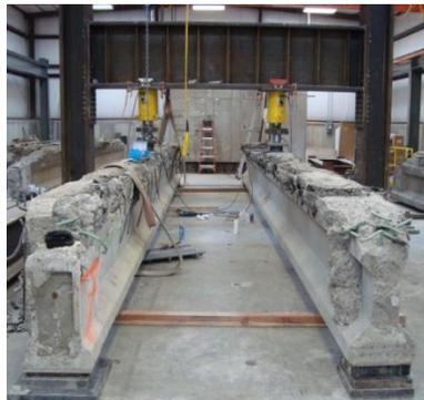
Figure 8 Set up with the reaction frame and two girders
