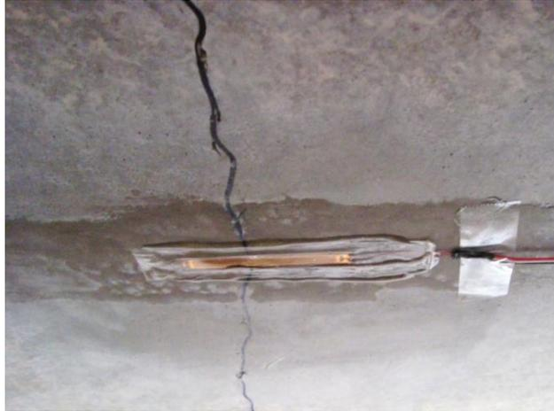
Figure 12 Strain gauge attached across the crack on bottom of girder
