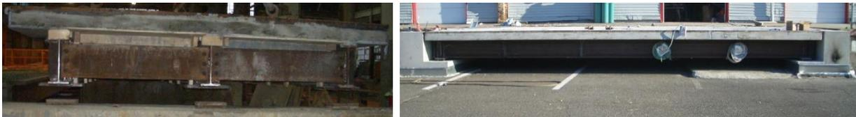
Figure 2. Left: The cross-section of the large scale composite bridge specimen in factory. Right: The bridge specimen simply supported on permanent supports [8].
