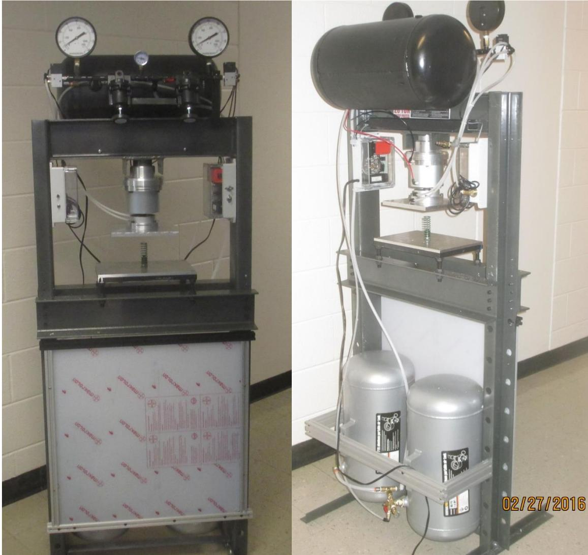
**Figure 32 - Pneumatically operated press frame load applicator press unit**
