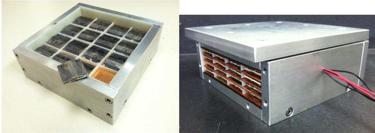
**Figure 8 - The transducers are arranged inside of an energy harvesting module.**
