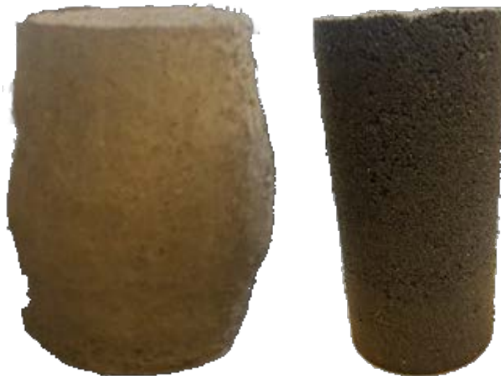
Figure 19 Specimen after (left) and before (right) shearing
