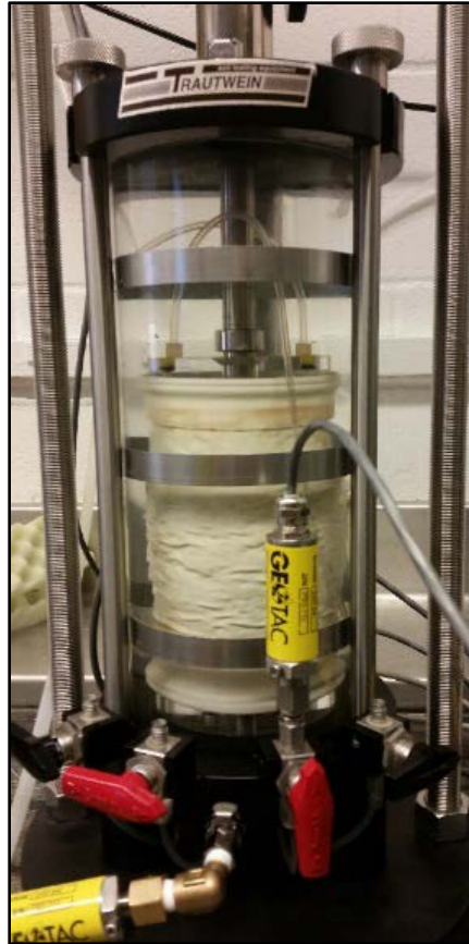
Figure 18 Failed specimen in loading frame
