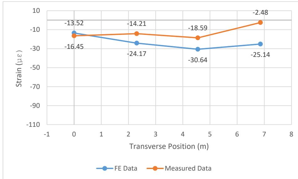
Figure 4.25 Transverse Strain Distribution for Top Flanges in Load Path Y3
