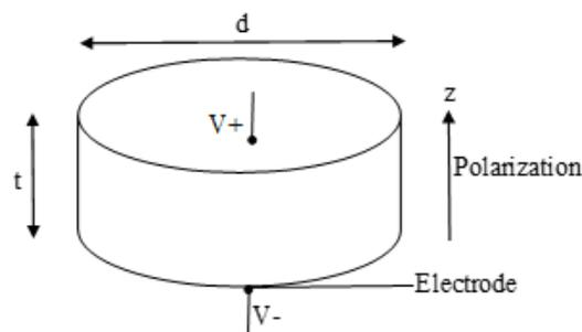
Figure 2 Illustration of disk/rod shaped PZT transducer
