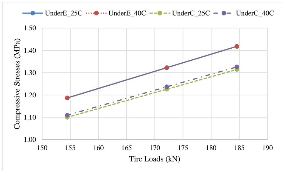
Figure 7 Compressive stresses under different tire loads at 8 km/h
