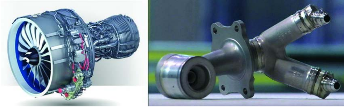
Figure 12 The LEAP engine (a) has 19 3D-printed fuel nozzles (b) (Mouzakis 2018).
