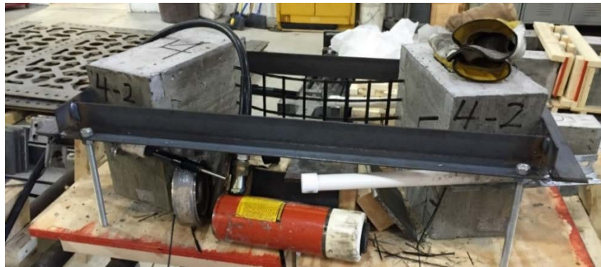
Figure 14. Typical Failure of a Development Length Specimen
