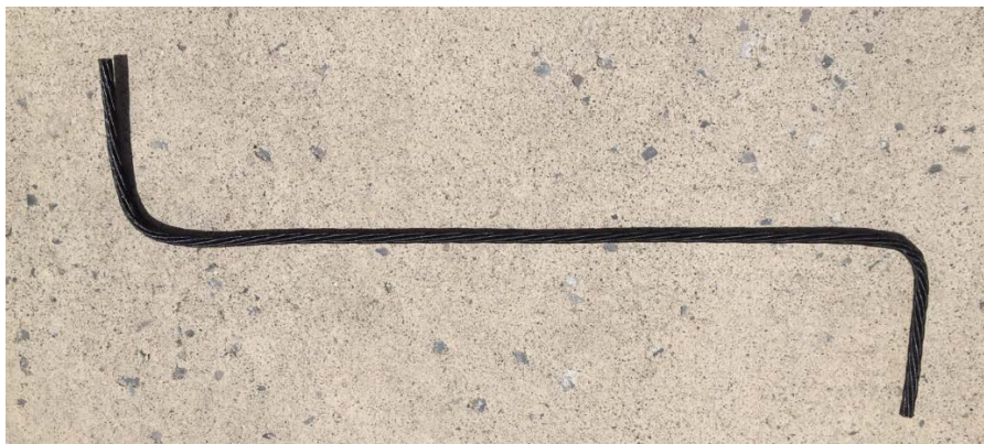
Figure 1. Typical CFCC Stirrup
