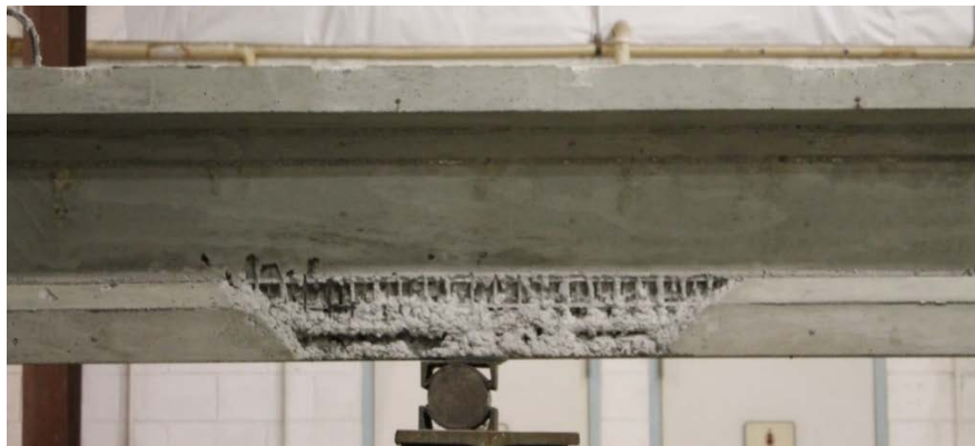
Figure 18. Honeycombing in Three Layers of C-Grid
