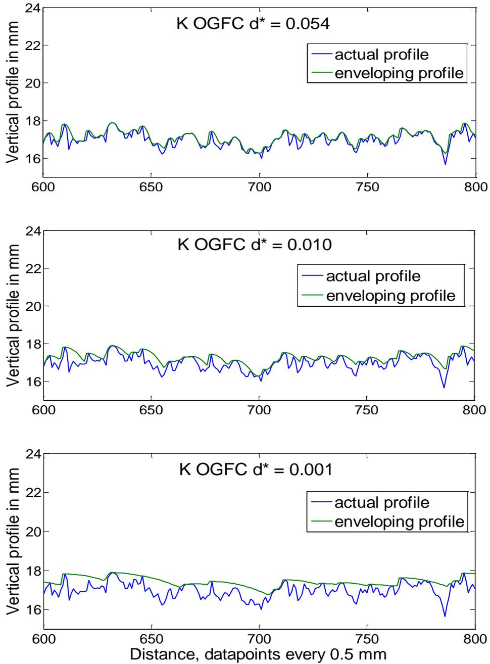
**FIGURE 7** Enveloping profile illustration calculated for different tire stiffnesses for a porous asphalt mix (e.g., 100 mm for Section K - OGFC).
