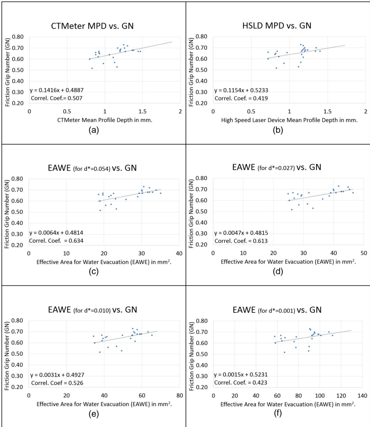
**FIGURE 9 Macrotexture vs. friction - correlations.**
