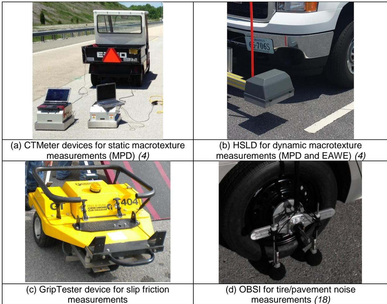
**FIGURE 3** Equipment used for the analysis.
