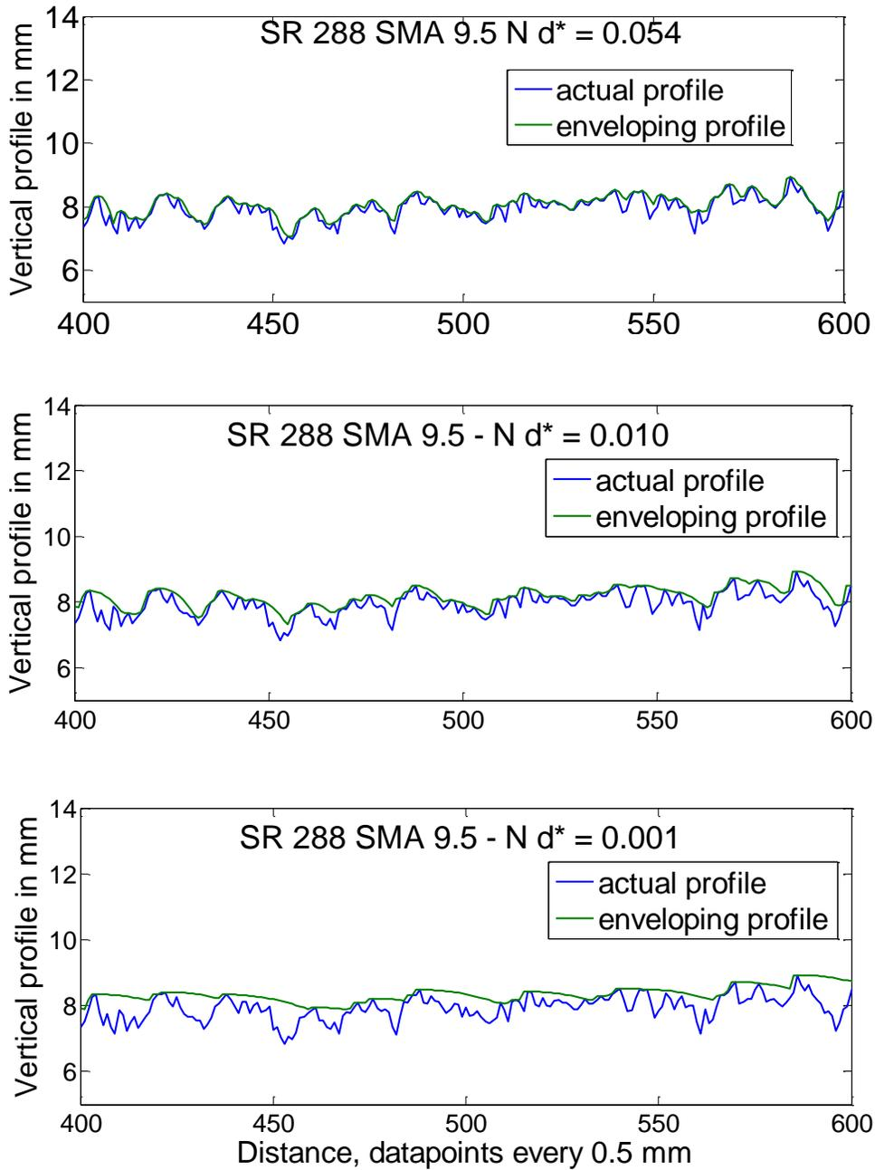
**FIGURE 6 Enveloping profile illustration calculated for different tire stiffnesses for a gap-graded asphalt mix (e.g., 100 mm for Section SR-288 SMA 9.5 N).**
