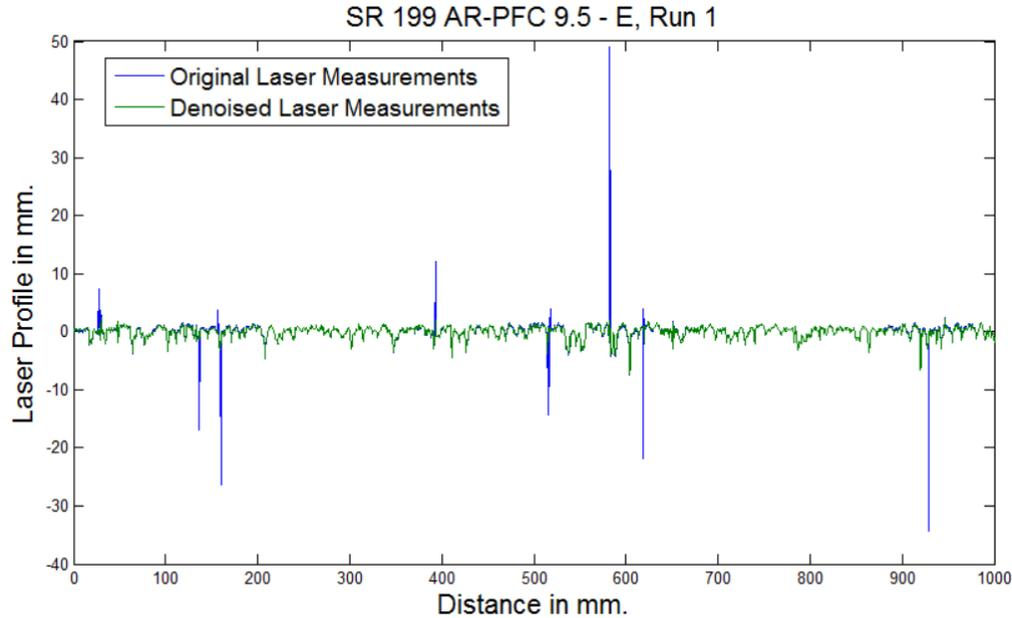
**FIGURE 5 HSLD Measurements, with and without spikes (1st meter of Section B-SM-9.5D).**
