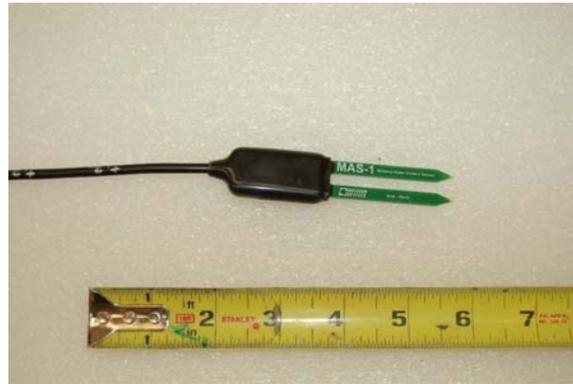
**Figure 3.13 Volumetric water content sensor**
