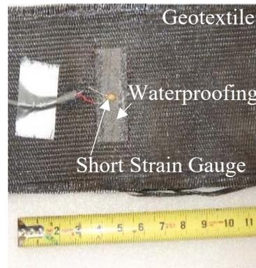
**Figure 3.8b Short strain gauge**
