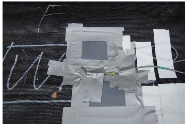
**Figure 3.12 Thermistor installation**
