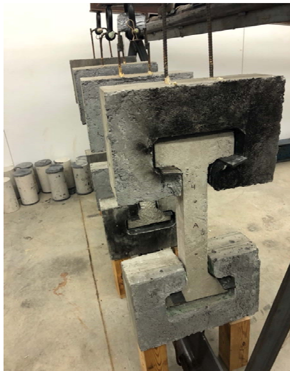
Figure 3-3: Tensile Creep Specimen Loaded
