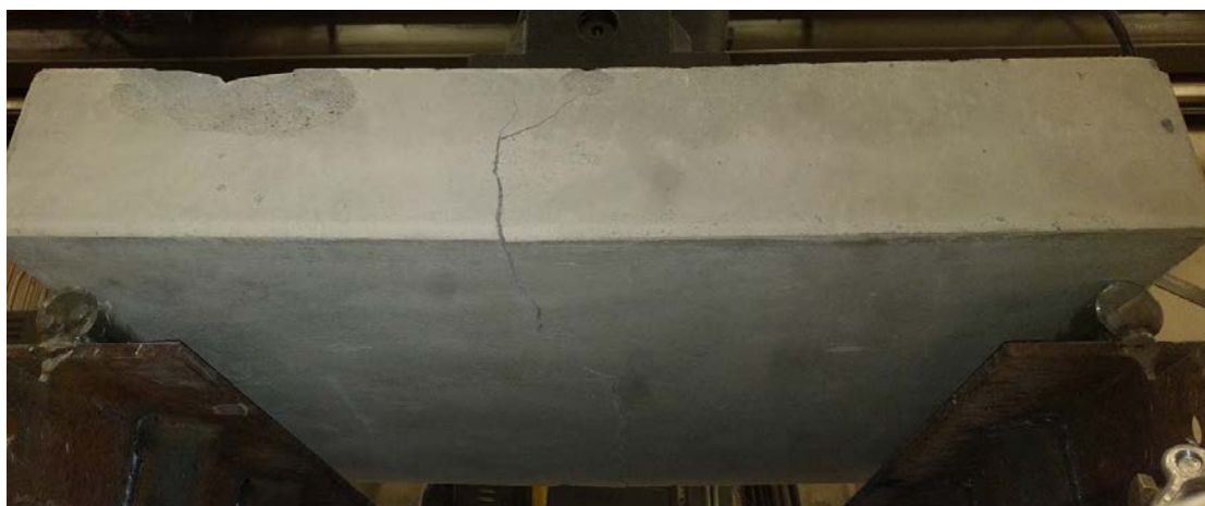
Figure 4.14 Crack 1/4 inch wide, load increased (32,000 cycles)
