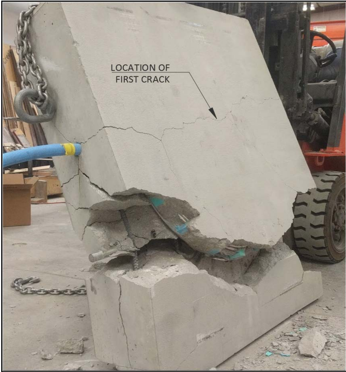
Figure 4.27 Third pad post failure
