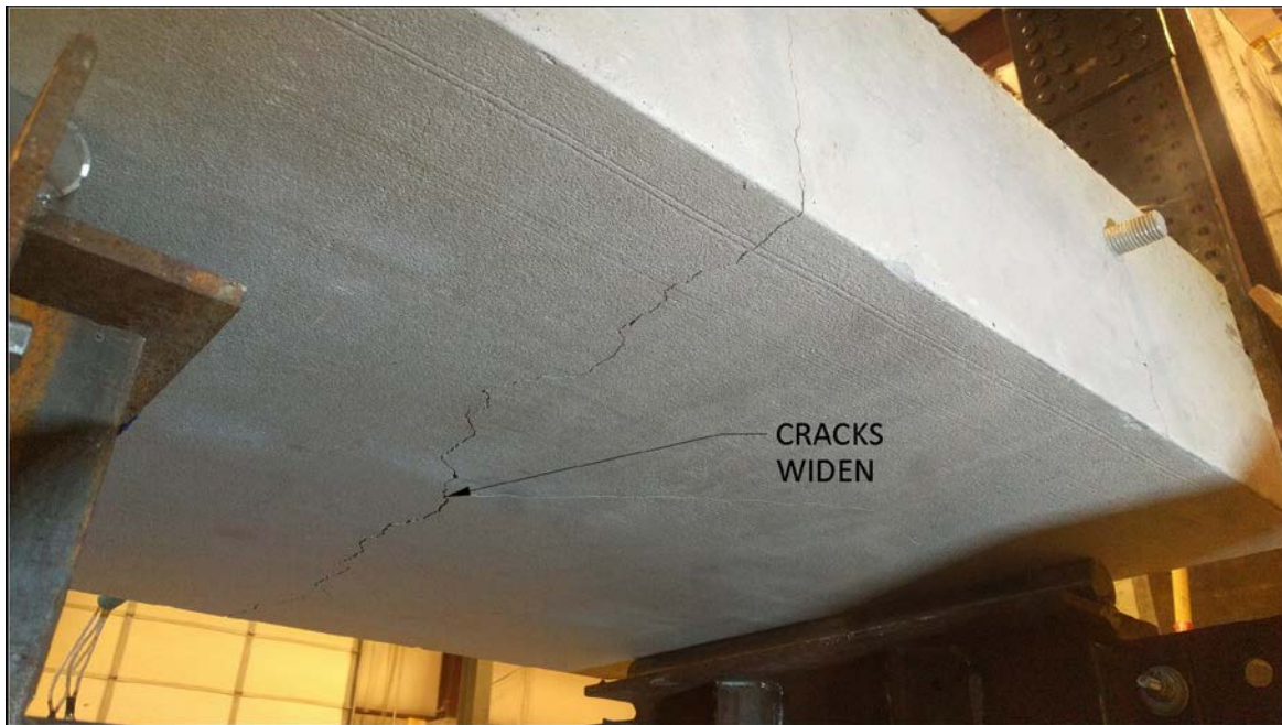
Figure 4.23 Crack 1/8 inch wide
