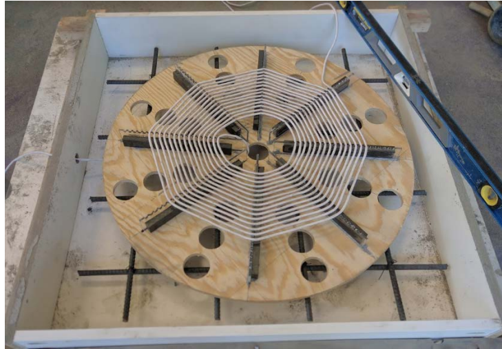
Figure 2.18 Test 3 IPT coil without aluminum plate
