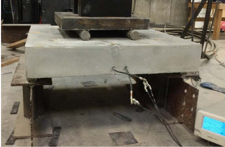
Figure 4.28 Other Sample tested with four-point bending test
