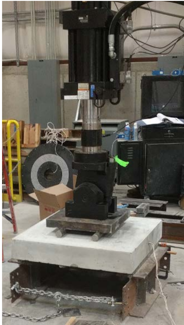
Figure 3.5 Four-point bending test set up
