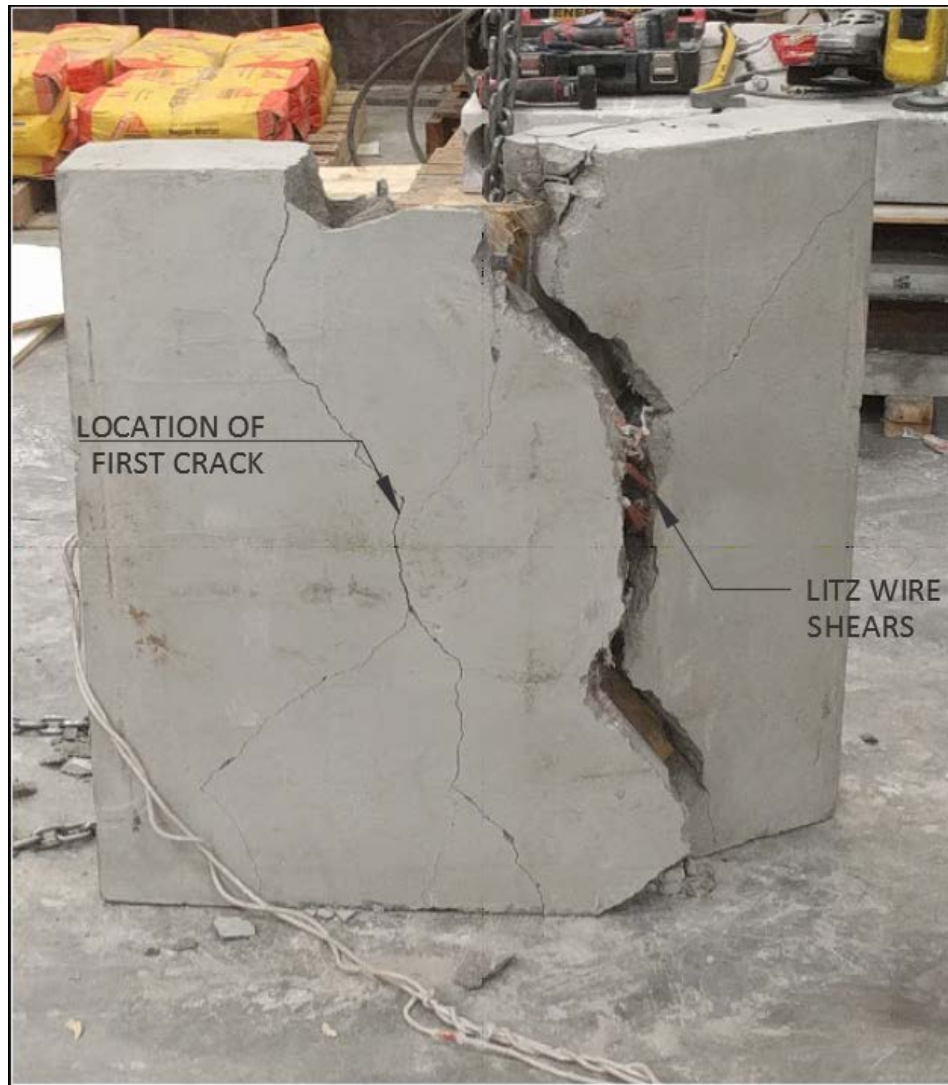
Figure 4.9 First pad post failure
