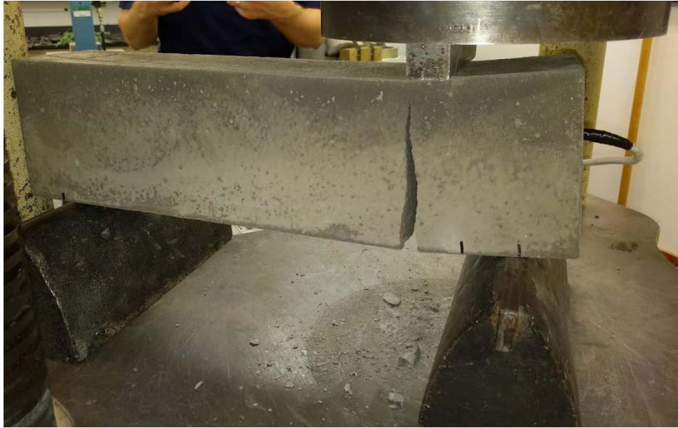
Figure 2.10 Concrete sample after failure
