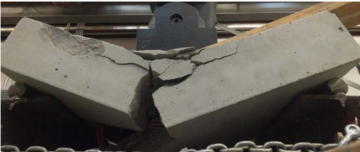
Figure 4.17 Failure (approximately 40,000 cycles)
