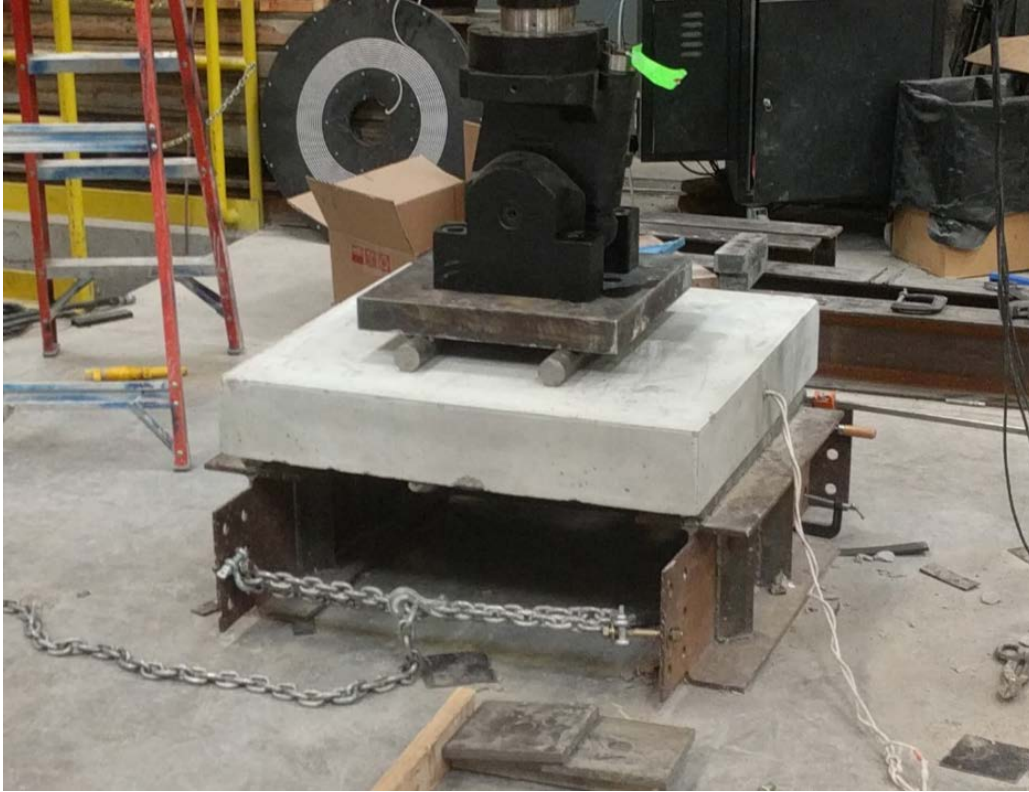
Figure 4.1 First fatigue test set-up
