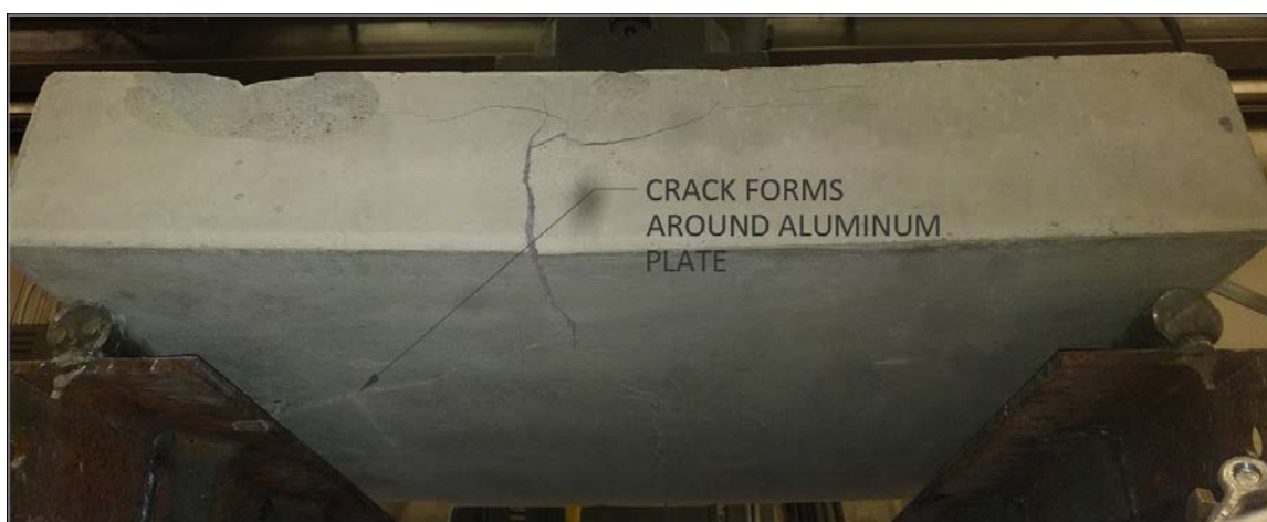
Figure 4.15 Crack 3/8 inch wide, (35,000 cycles)
