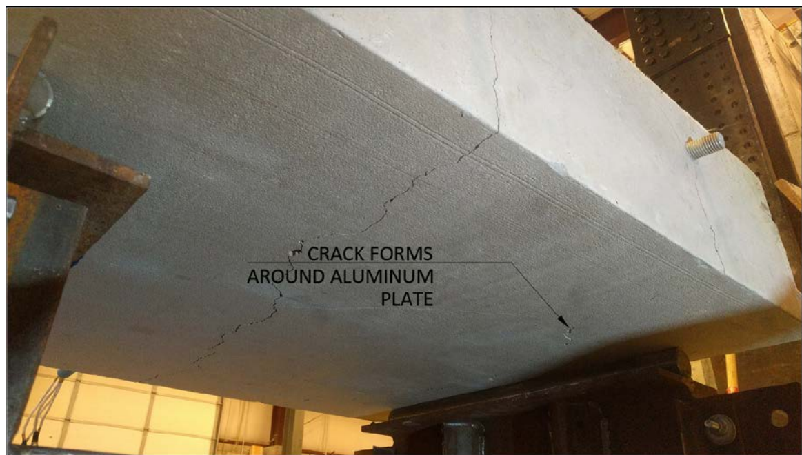
Figure 4.24 Crack 1/4 inch wide
