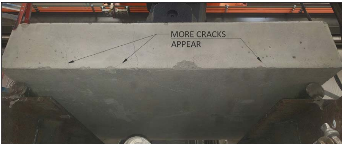
Figure 4.6 Load was increased to 9000 lbs. (approximately 20,000 cycles)
