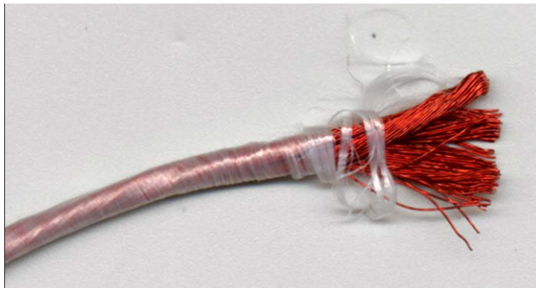
Figure 2.16 Litz wire with nylon sheathing
