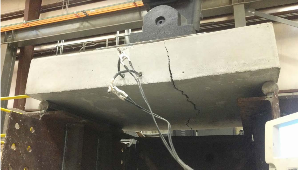
Figure 4.29 Other sample after failure
