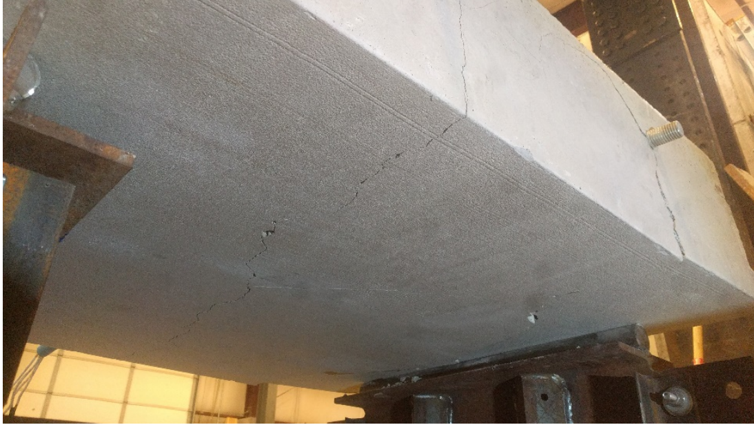
Figure 4.25 Crack 1/2 inch wide
