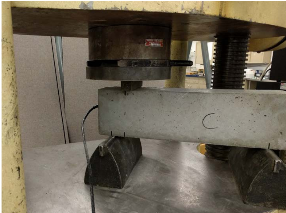
Figure 2.9 Break test set-up
