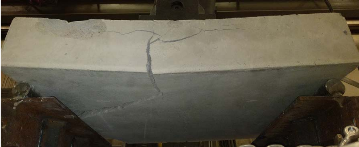
Figure 4.16 Crack \frac{3}{4} inch wide, (36,000 cycles)
