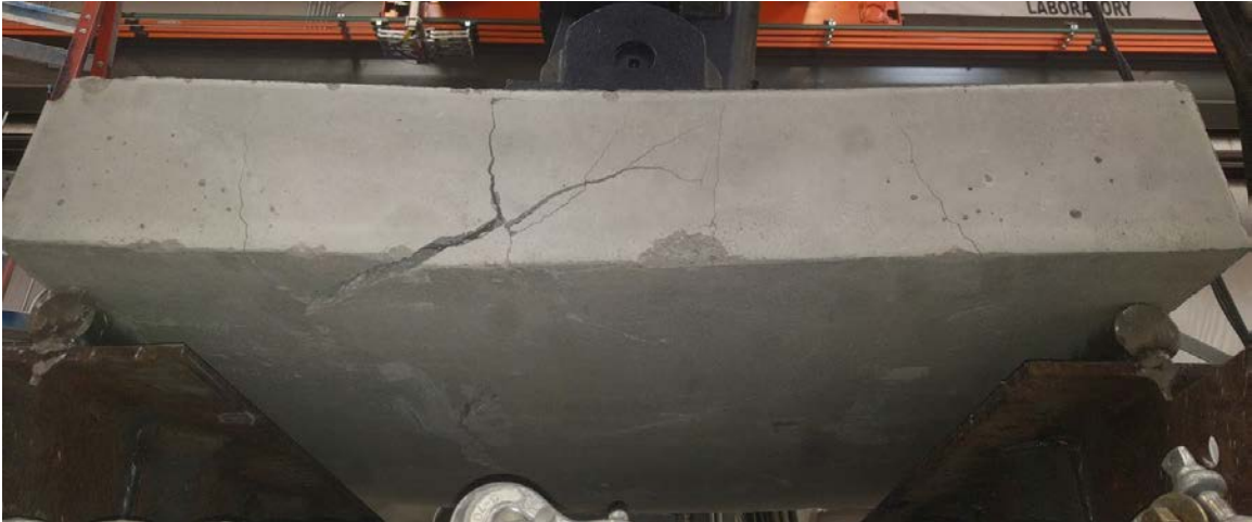
Figure 4.7 Cracks 1/2 inch (approximately 25,000 cycles)
