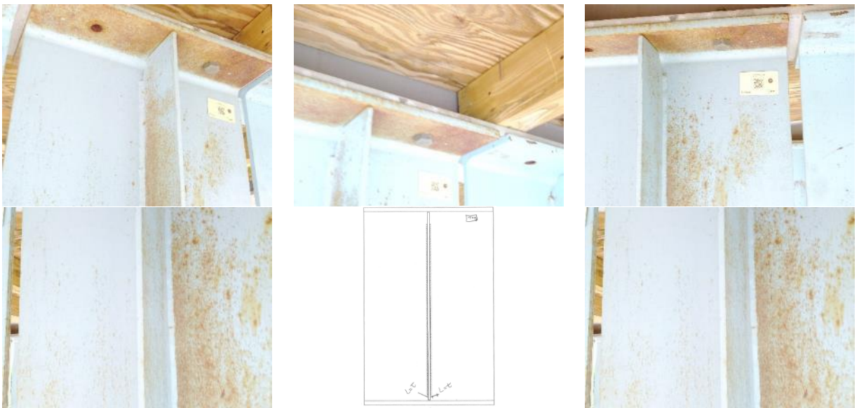
Figure 6.12 Postmortem result and inspection pictures of crack-free specimen
