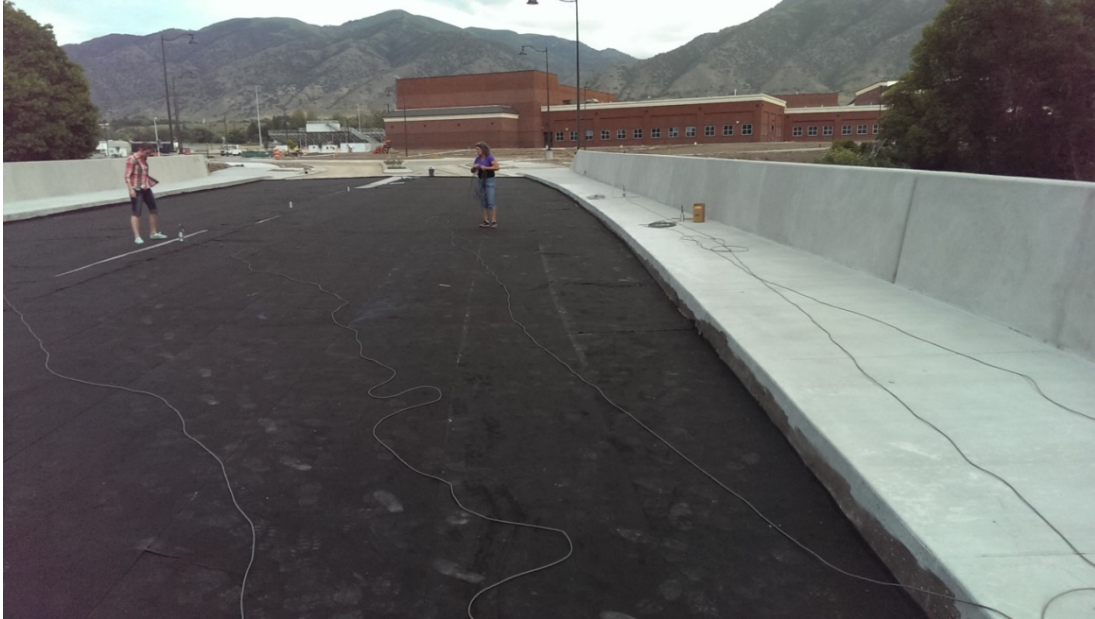
Figure 3.1: Preparing Sensors for the Impact Test
