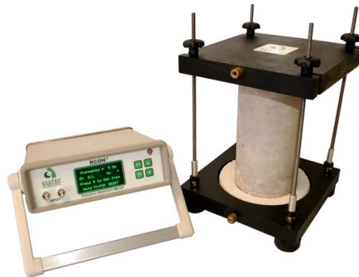
Figure 2.7 Giatec Scientific Inc. instrument for measuring Bulk resistivity
