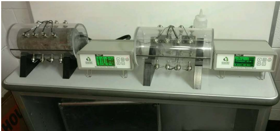
Figure 3.9 Inter-laboratory investigation with USU and UDOT surface electrical resistivity machine
