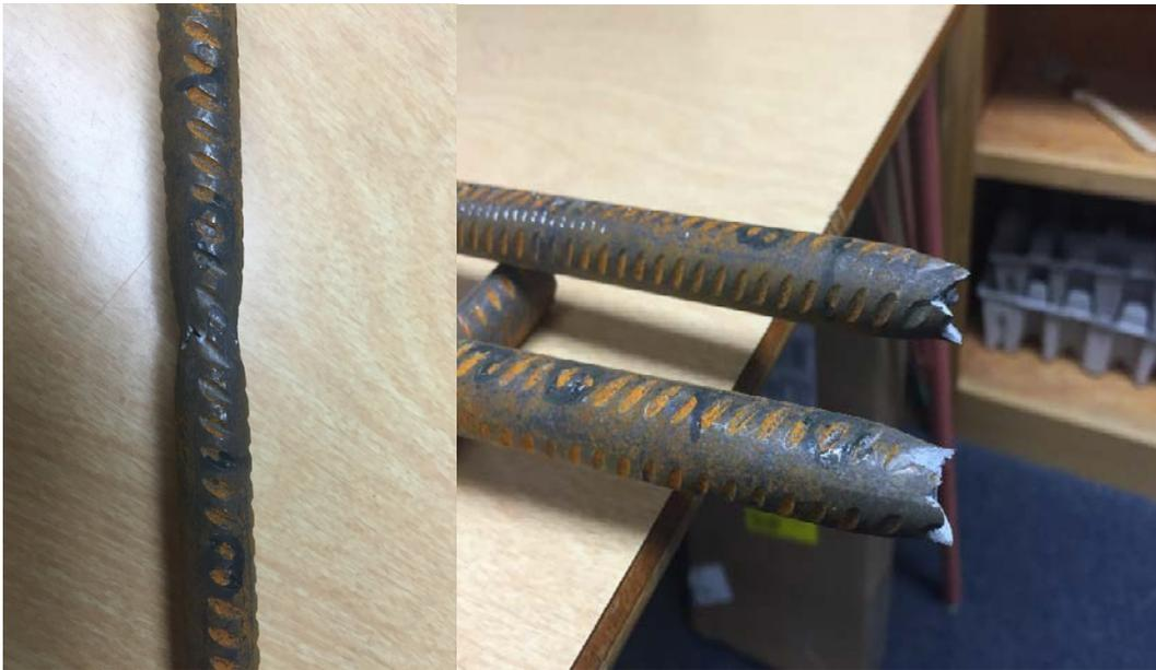
*Figure 3.6 Ductile failure mode in free wire of Black (none-coated) wire*
