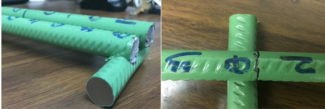
*Figure 3.5 Brittle failure at cross weld in epoxy coated wire*
