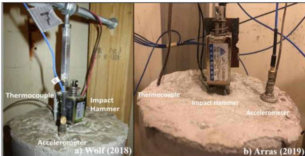
Figure 3.3 Seismic Modulus and Internal Temperature Monitoring
