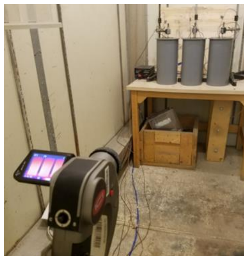
Figure 3.9 Set-up for Thermal Imaging of Cylinders
