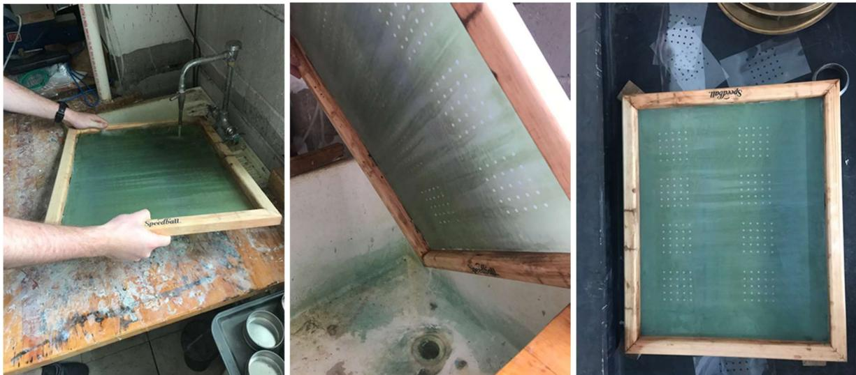
**Figure 2.7 Screen washing after light exposure.**
