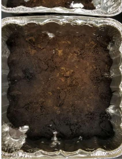
**Figure 6.5 Charred shredded cotton and polyester recycled textiles after attempted thermal bonding.**
