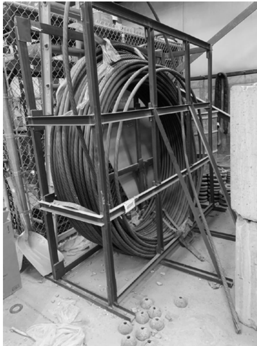
Figure 1-3 1-1/8 in. diameter strand in 6.5 ft diameter spool.
