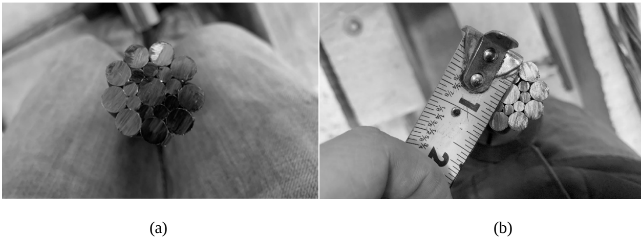
Figure 1-1 1-1/8 in. diameter strand (a) Cross Section (b) Measurement of Cross Section
