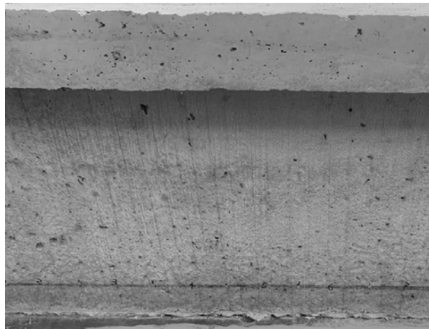
Figure 3-13 Caliper marks mounted on beam at the level of the strand
