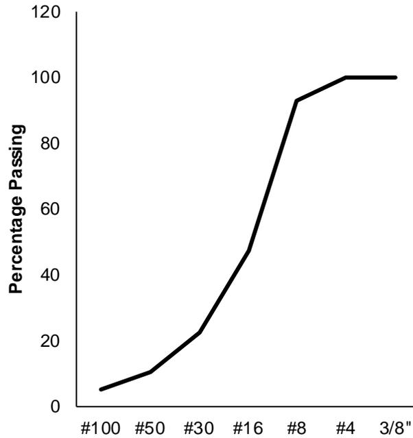
Figure 3.5 Lightweight crushed fines gradation
