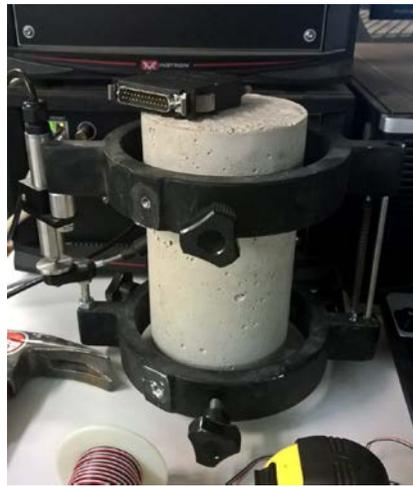
Figure 3.7 Compressometer for determination of modulus of elasticity (ASTM C469)
