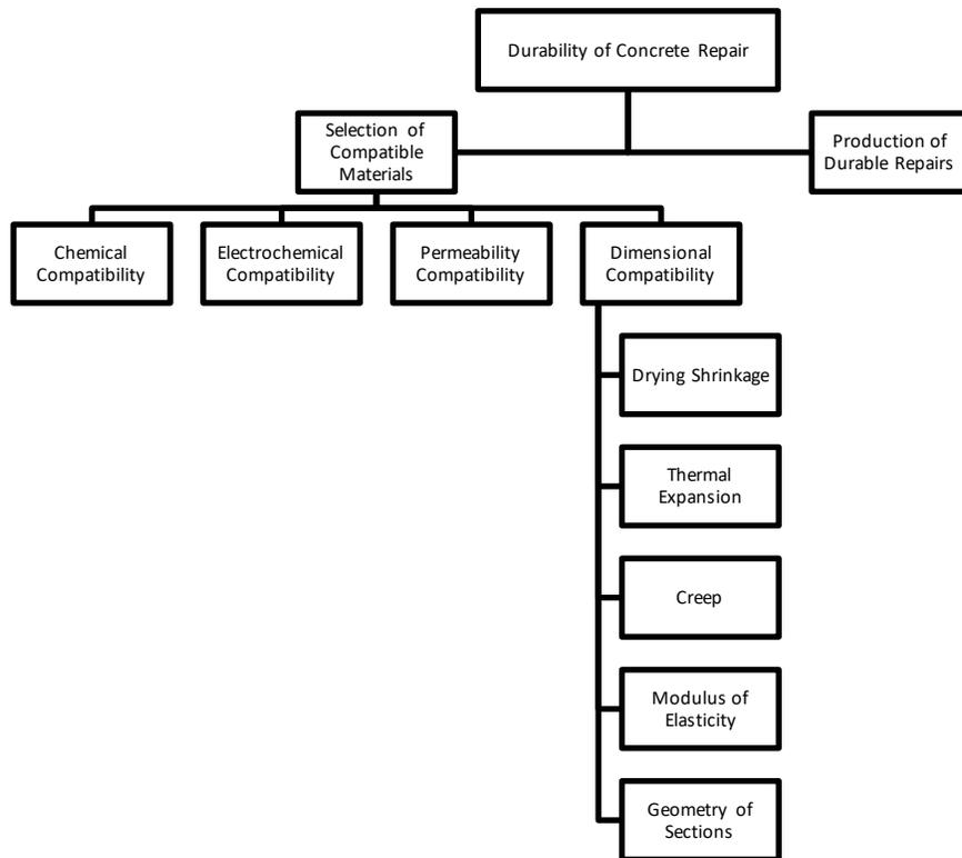
**Figure 2.1 Factors affecting durability of concrete repairs (Adaptation from Emmons et al)**
