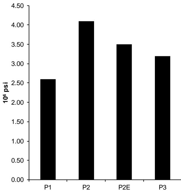
Figure 4.2 Modulus of elasticity of proprietary materials (age = 4 hours)
