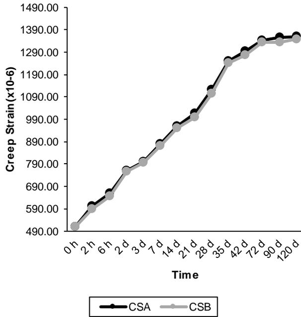
Figure 4.19 Creep shrinkage for OPCIC
