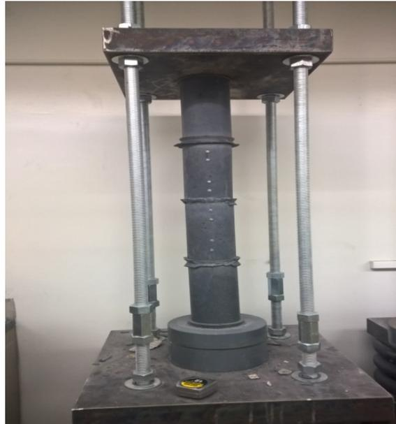
**Figure 3.12 Creep testing frame (ASTM C512)**
