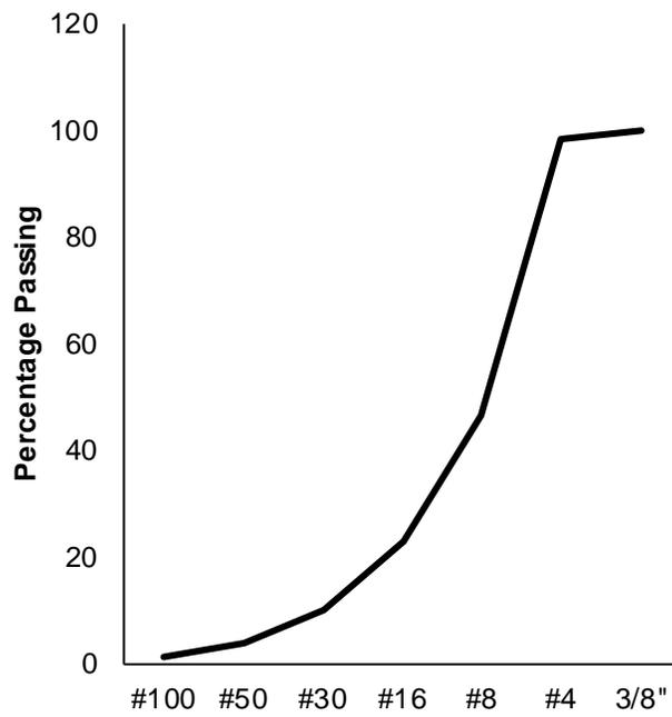
Figure 3.4 Lightweight fine aggregate gradation
