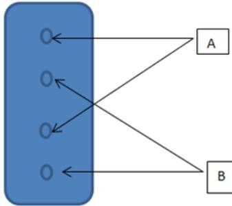
**Figure 3.11 Reference measurement locations for creep shrinkage strain**
