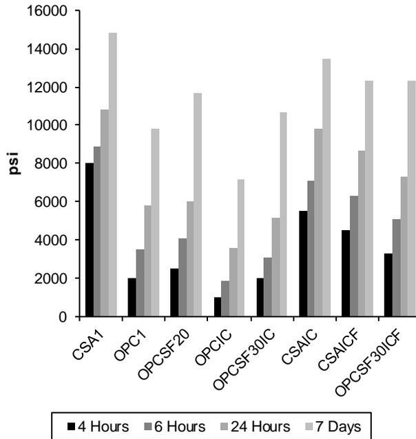
**Figure 4.9 Compressive strength of Phase II non-proprietary repair media**
