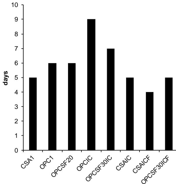
**Figure 4.15 Time to first crack in restrained ring shrinkage tests of Phase II mixtures**
