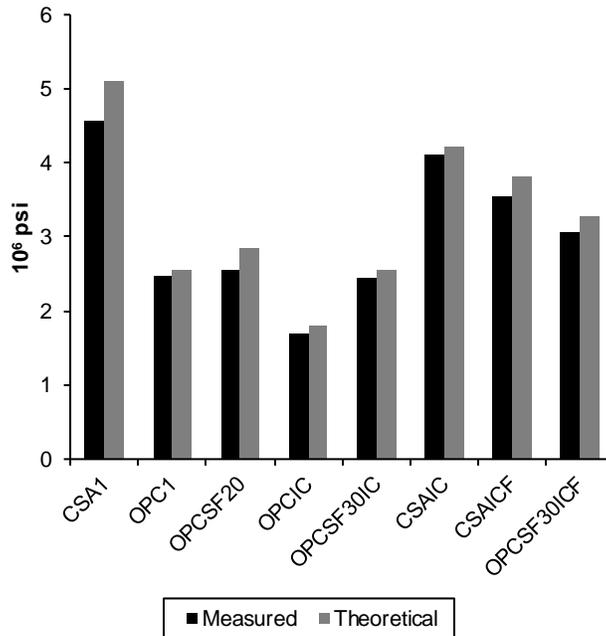
Figure 4.10 Predicted and measured moduli of elasticity of Phase II non-proprietary repair media
