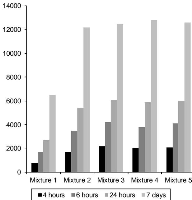
**Figure 4.8 Type III Compressive Strengths**
