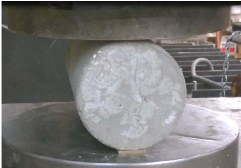
Figure 3.8 Splitting tensile (Brazilian) test (ASTM C496)
