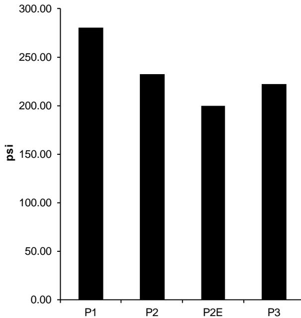
Figure 4.3 Splitting tensile strength of proprietary materials (age = 4 hours)
