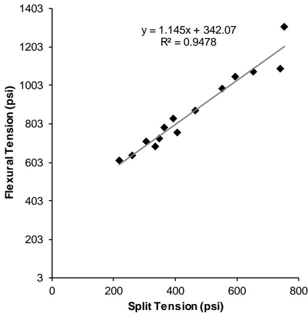
Figure 4.12 Fitted data to a linear regression equation with an R square value of 0.94 from Split Tensile and Flexural Strength data
