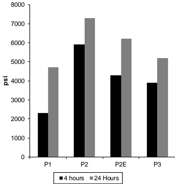
Figure 4.1 Compressive strength of proprietary materials (age = 4 and 24 hours)
