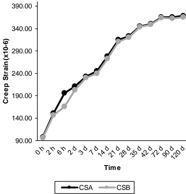
Figure 4.18 Creep shrinkage for OPCSF20
