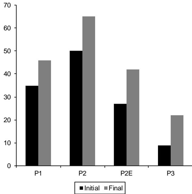
Figure 4.5 Initial and Final setting times (min) of proprietary materials
