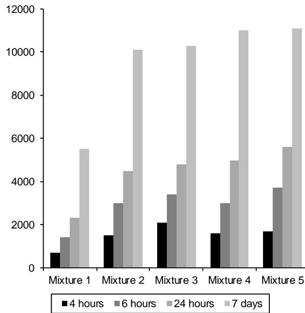
**Figure 4.6 Type II/V Compressive Strengths**
