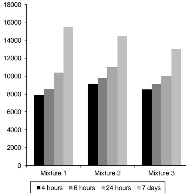
**Figure 4.7 CSA Compressive Strengths**
