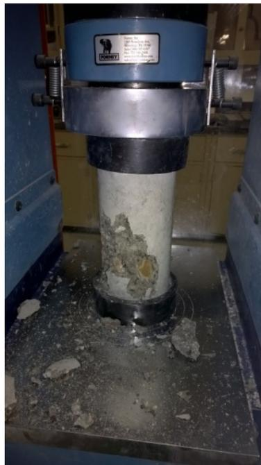
Figure 3.6 Cylinder in the compression test with neoprene caps
