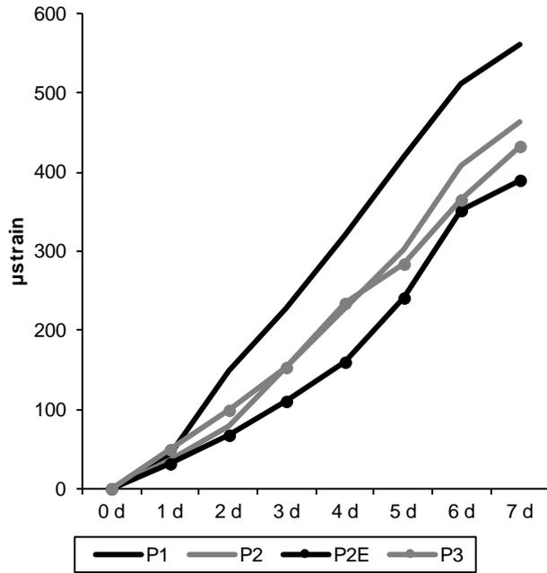
Figure 4.4 Drying Shrinkage Strain for proprietary materials
