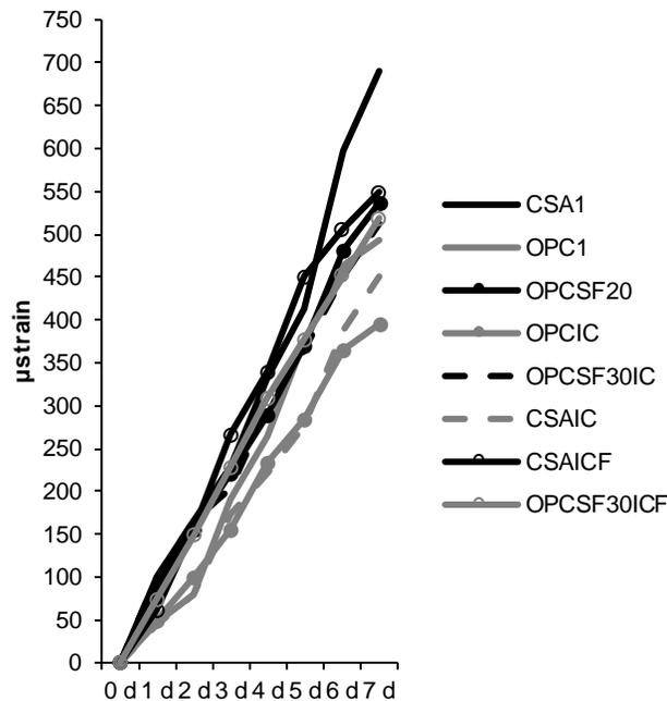
Figure 4.14 Drying shrinkage in Phase II mixtures
