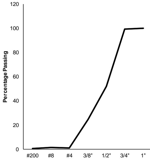
**Figure 3.1 Normalweight coarse aggregate gradation**
