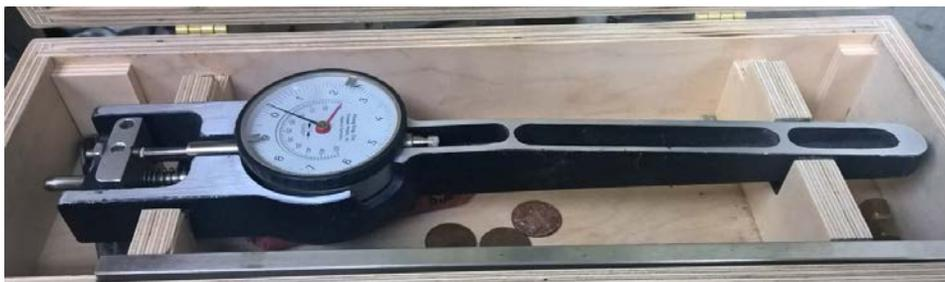
**Figure 3.13 Creep strain gauge**
