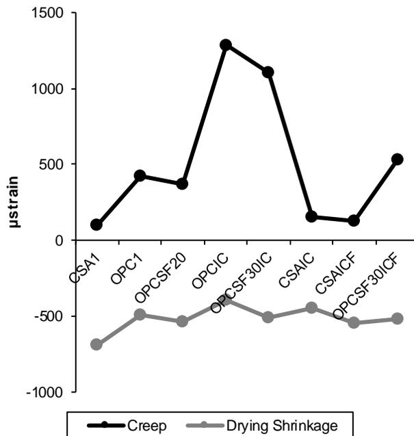
Figure 4.24 Length Change and Max Creep per Mixture in Microstrain
