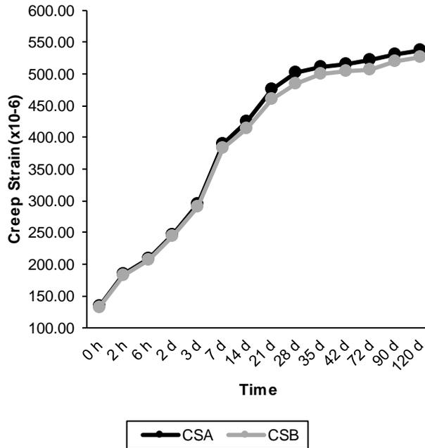
**Figure 4.23 Creep shrinkage for OPCSF30ICF**
