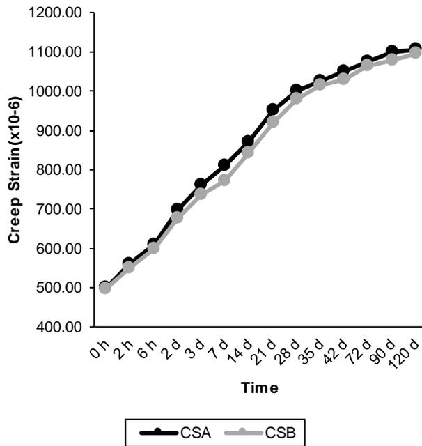
Figure 4.20 Creep shrinkage for OPCSF30IC
