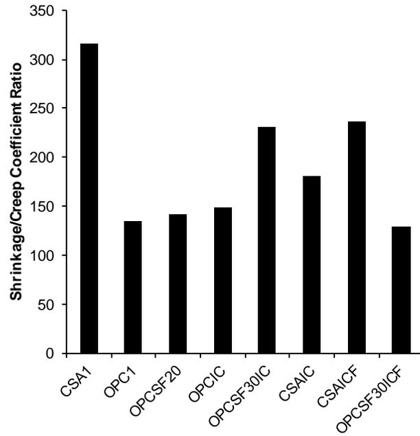
Figure 4.25 Shrinkage/Creep Coefficient Ratio
