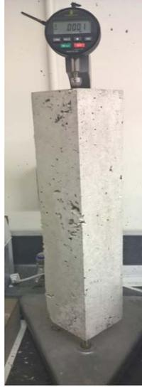
**Figure 3.9 Length comparator (ASTM C157)**
