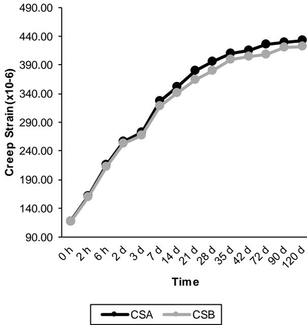
Figure 4.17 Creep shrinkage for OPC1
