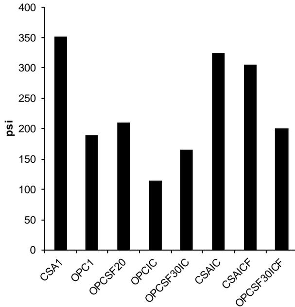
Figure 4.11 Splitting tensile strength of Phase II non-proprietary repair media
