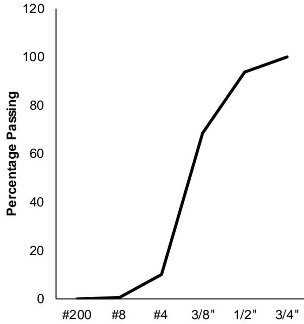
Figure 3.3 Lightweight coarse aggregate gradation
