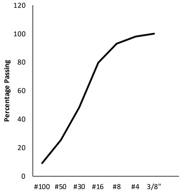
**Figure 3.2 Normalweight fine aggregate gradation**
