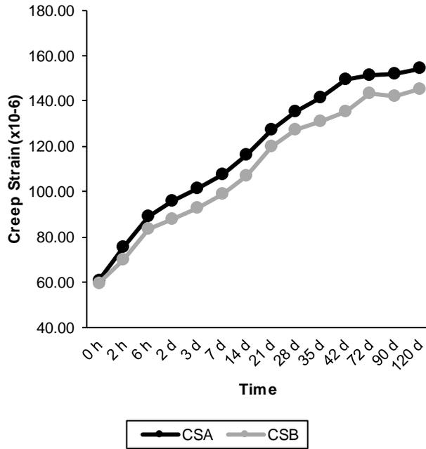
Figure 4.21 Creep shrinkage for CSAIC
