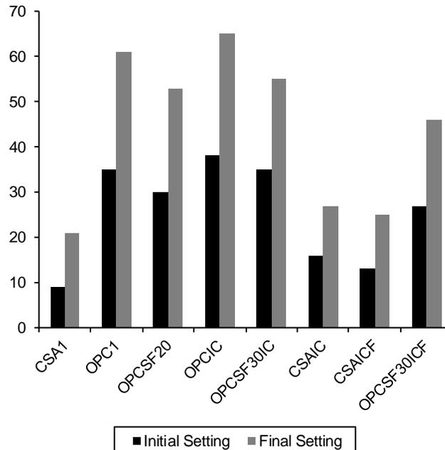
Figure 4.13 Initial and final setting times of Phase II non-proprietary repair media
