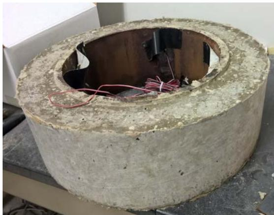
Figure 3.10 Restrained ring shrinkage test (ASTM C1581)
