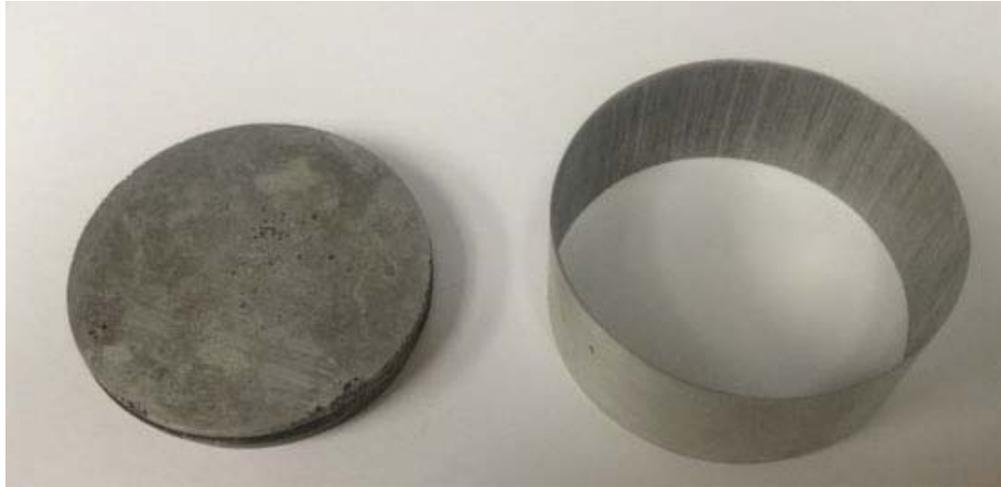
Figure 16- Cutting Ring and Base Puck
