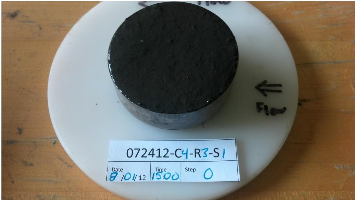
Figure 18- Completed Sample With Ring and Puck
