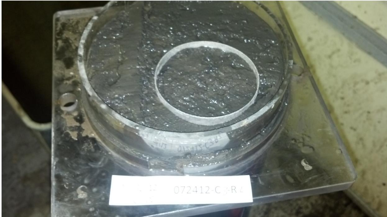
**Figure 17- Extruded Sample with Cutting Ring**
