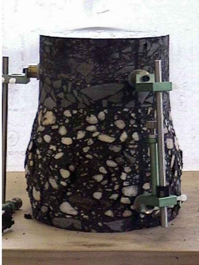
Figure 19 – Failed Sample During 130°F Test Temperature
