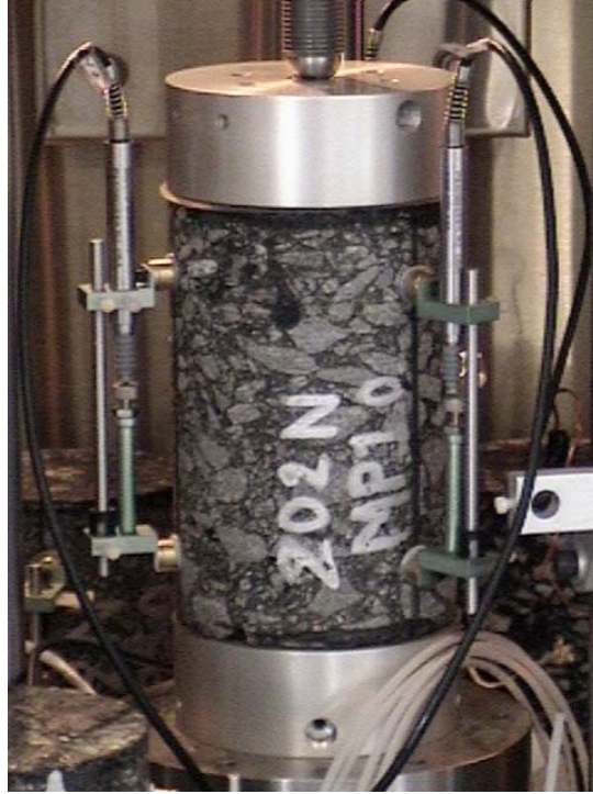
Figure 22 – Dynamic Modulus Sample from NJ Route 202 Prior to Testing
