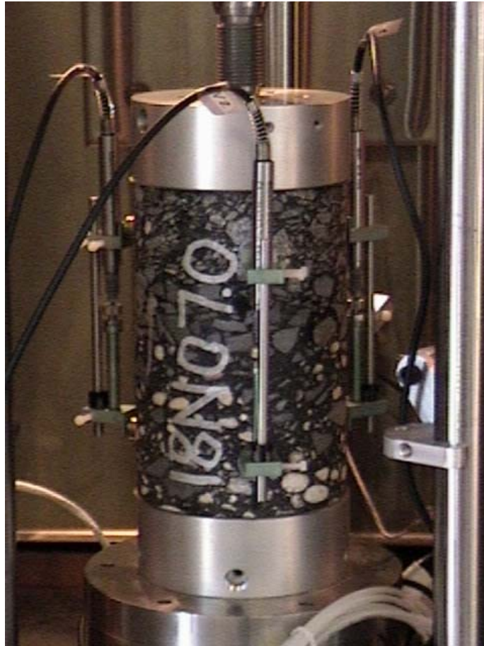
Figure 2 – HMA Sample Instrumented for the Dynamic Modulus Test
