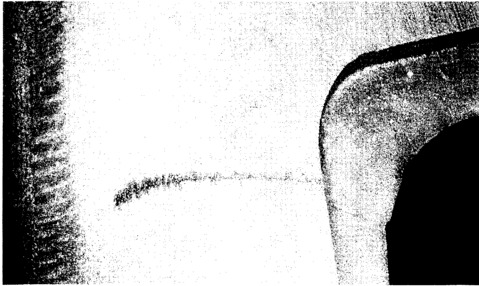
Figure 3-13 Fatigue Crack in Transformer Base of Specimen S-3
