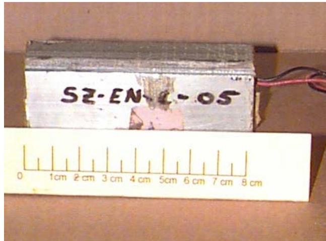
Figure 4: (b) Photograph of the final sensor assembly ready for loading tests.
