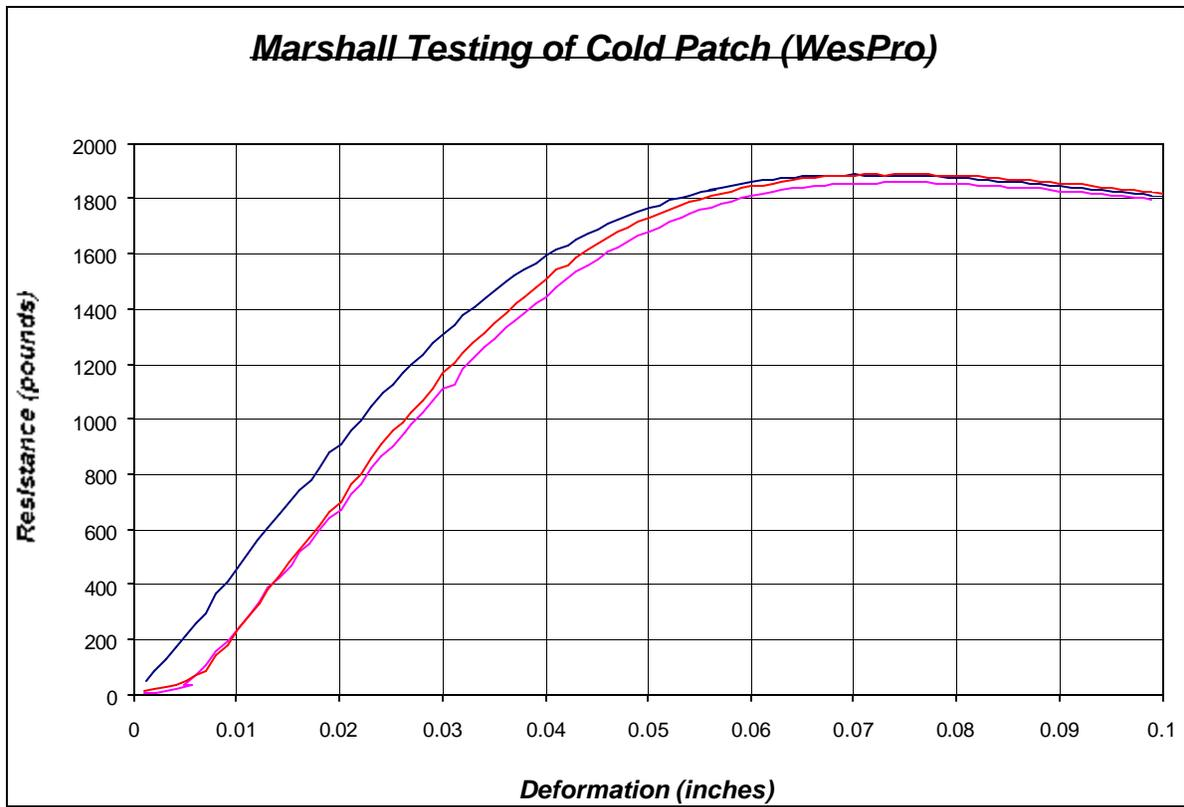
**Figure 29. Marshall Testing of Cold patch (WesPro)**
