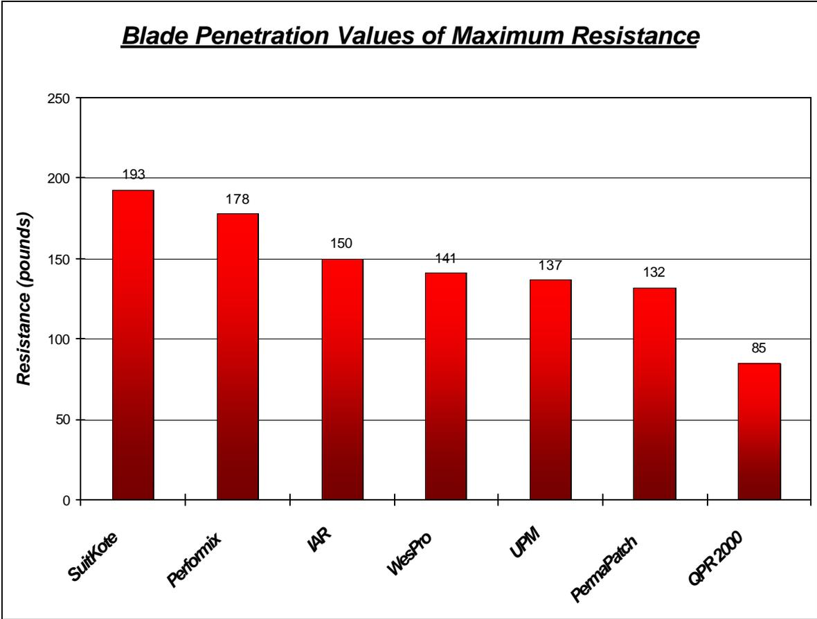
**Figure 30. Blade Penetration Values of Maximum Resistance**
