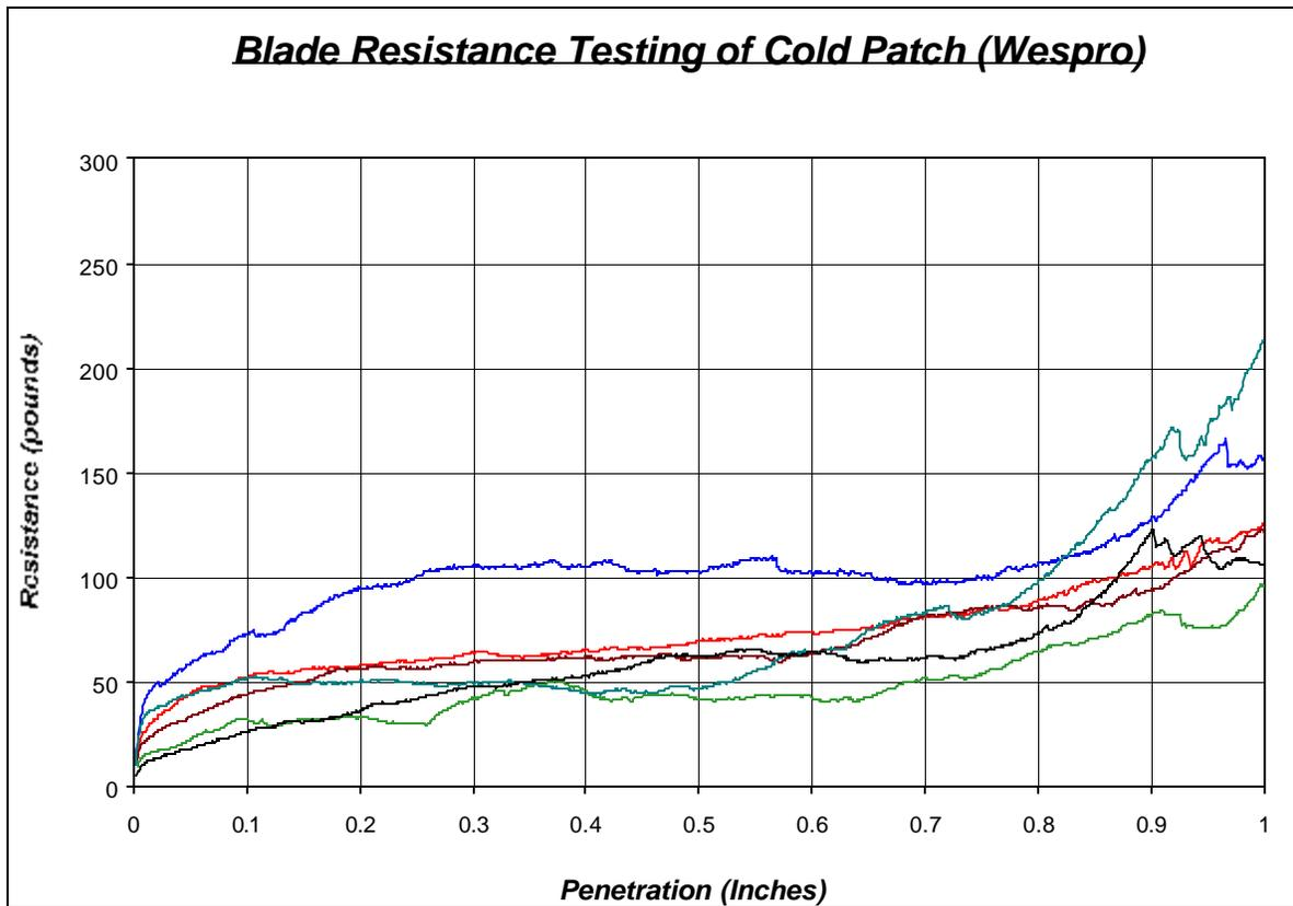
**Figure 37. Blade Resistance Testing of Cold Patch (Wespro)**
