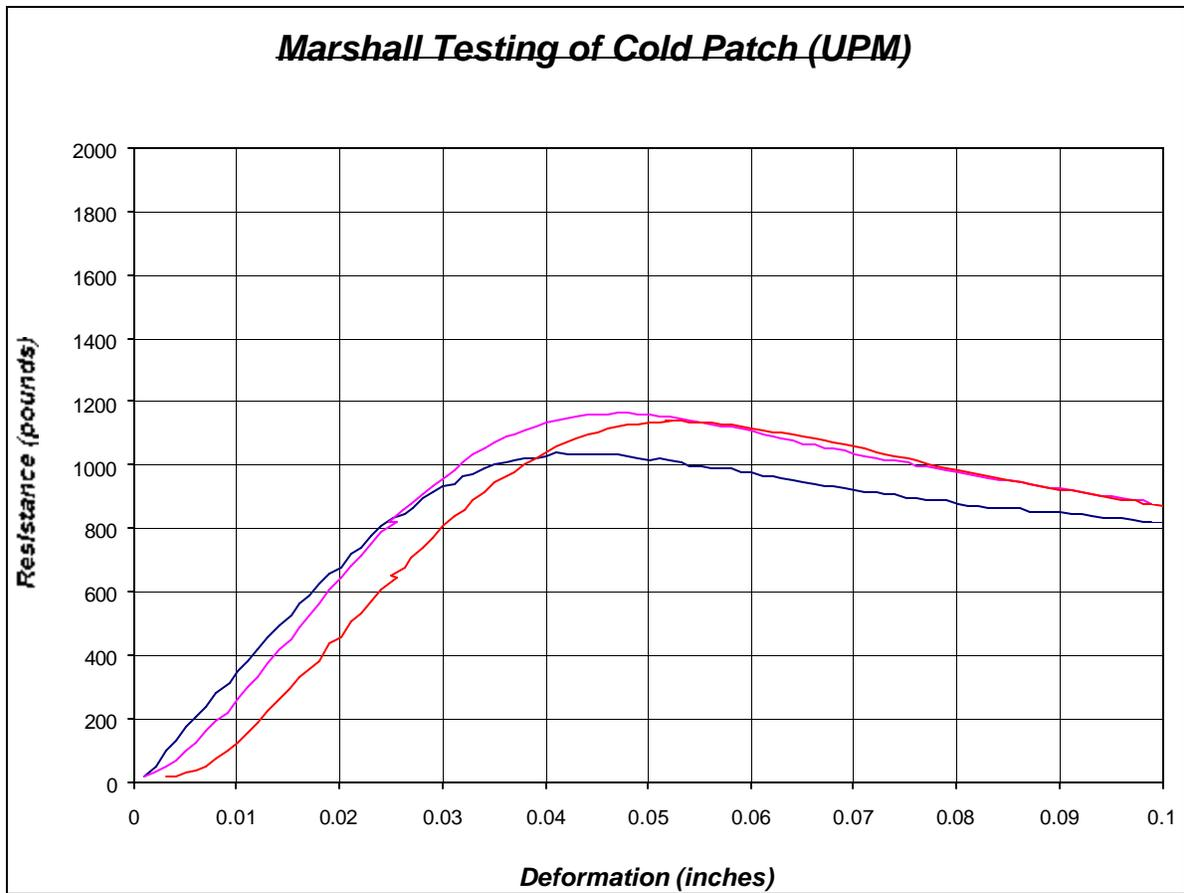
**Figure 28. Marshall Testing of Cold Patch (UPM)**
