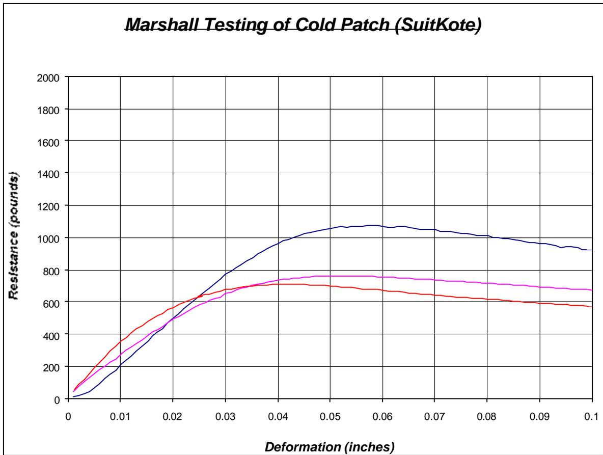
**Figure 27. Marshall Testing of Cold Patch (SuitKote)**
