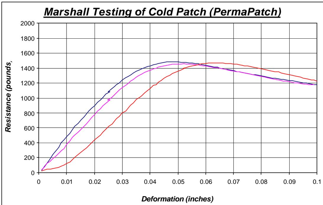
**Figure 25. Marshall Testing of Cold patch (PermaPatch)**
