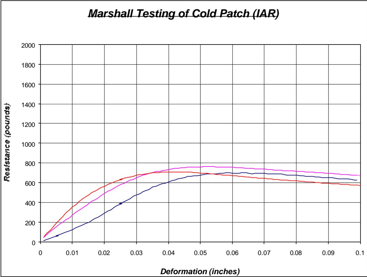
**Figure 23. Marshall Testing of Cold patch (IAR)**
