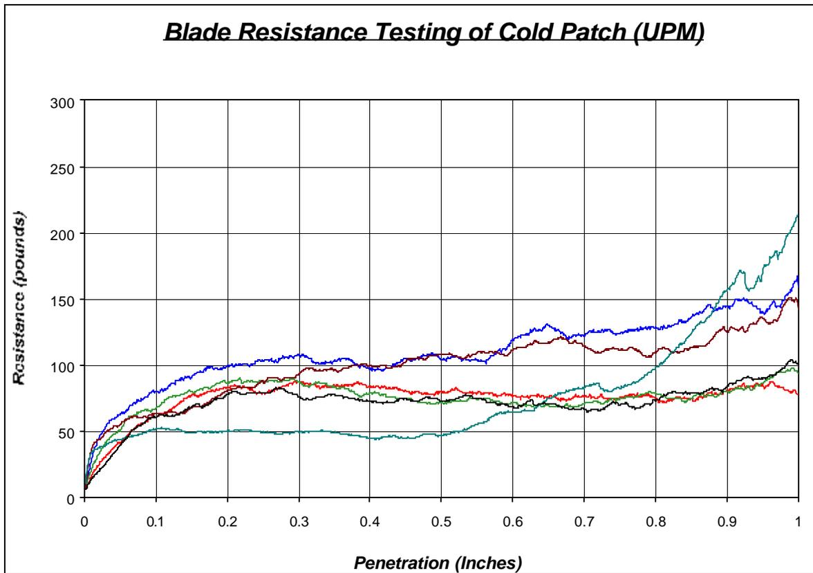
**Figure 35. Blade Resistance Testing of Cold Patch (UPM)**
