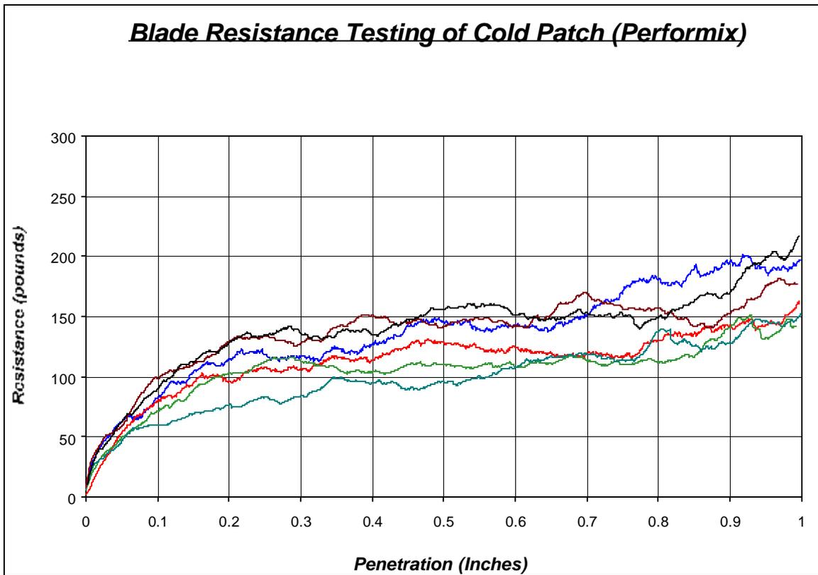
**Figure 32. Blade Resistance Testing of Cold Patch (Performix)**
