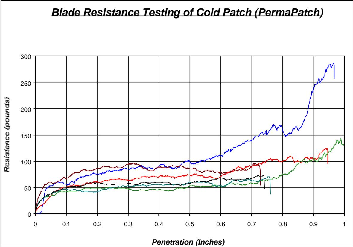
**Figure 33. Blade Resistance Testing of Cold Patch (PermaPatch)**
